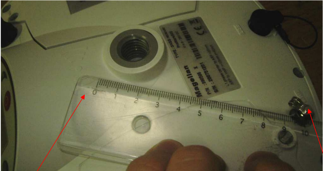
The distance between GSM and Bluetooth antennas is 10 cm
