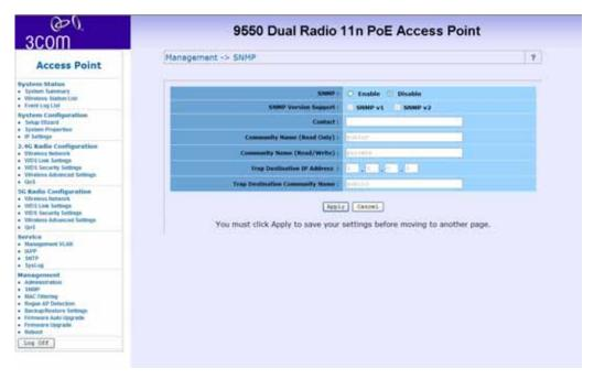
The SNMP administrative functions are changed through this section. The following functions can be changed:
