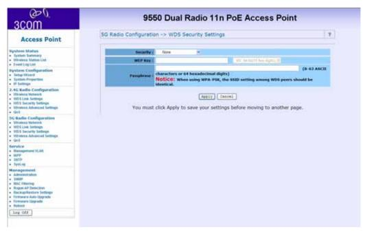
Choose the required security level from: **None, WEP, WPA-PSK (TKIP)**, **WPA-PSK (AES)**, **WPA2-PSK (TKIP)**, or **WPA2-PSK (AES)**.
