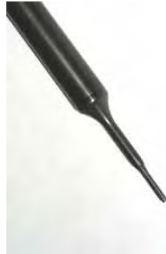
Fig. 5.2 EX3DV4 E-field Probe
