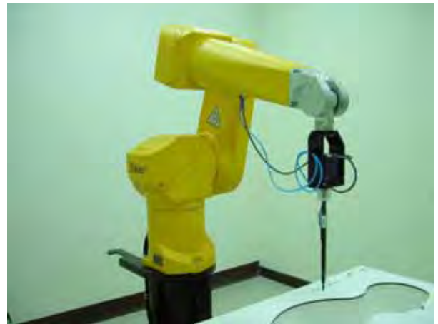
Fig. 5.2 Probe setup on robot
