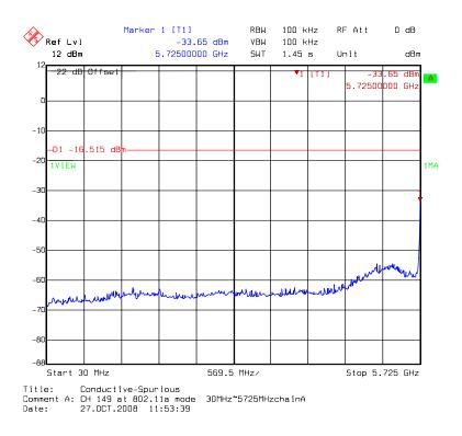
Chain A: conducted spurious @ 802.11a mode channel 149 (2 of 4)
