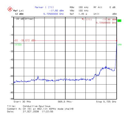
Chain B: conducted spurious @ 802.11n HT40 mode channel 151 (2 of 3)
