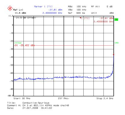
Chain B: conducted spurious @ 802.11n HT40 mode channel 3 (2 of 3)
