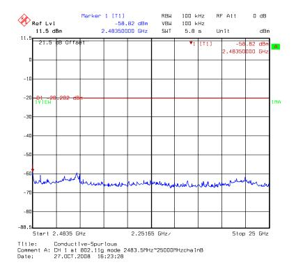
Chain B: conducted spurious @ 802.11g mode channel 6 (1 of 3)
