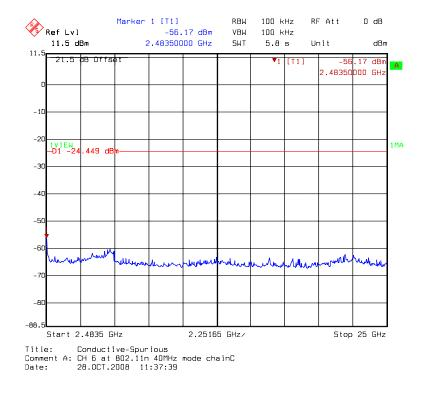
Chain C: conducted spurious @ 802.11n HT40 mode channel 9 (1 of 3)
