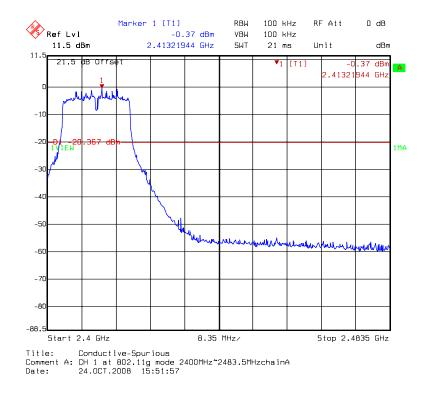
Chain A: conducted spurious @ 802.11g mode channel 1 (3 of 3)
