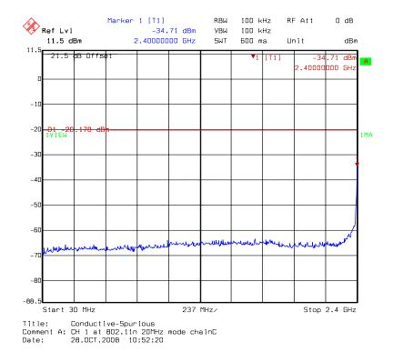
Chain C: conducted spurious @ 802.11n HT20 mode channel 1 (2 of 3)
