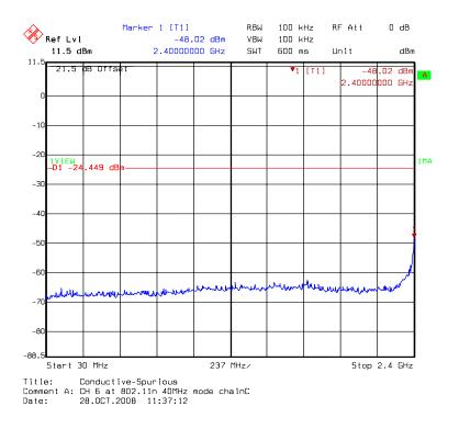
Chain C: conducted spurious @ 802.11n HT40 mode channel 6 (2 of 3)
