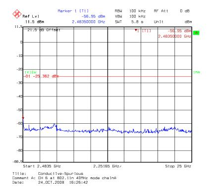
Chain A: conducted spurious @ 802.11n HT40 mode channel 9 (1 of 3)
