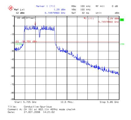
Chain A: conducted spurious @ 802.11n HT40 mode channel 151 (3 of 3)
