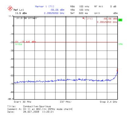
Chain C: conducted spurious @ 802.11n HT20 mode channel 11 (2 of 3)
