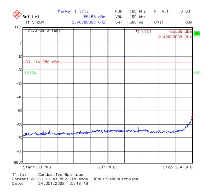
Chain A: conducted spurious @ 802.11b mode channel 11 (2 of 3)
