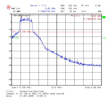
Chain B: conducted spurious @ 802.11n HT20 mode channel 149 (3 of 3)
