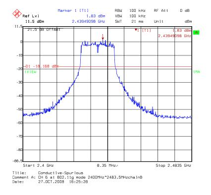
Chain B: conducted spurious @ 802.11g mode channel 6 (3 of 3)
