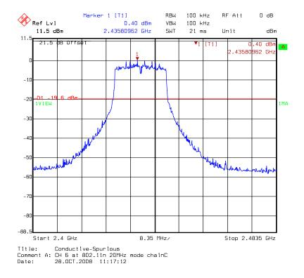
Chain C: conducted spurious @ 802.11n HT20 mode channel 6 (3 of 3)
