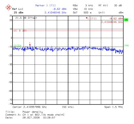
Chain C: Power Spectral Density @ 802.11b mode channel 6
