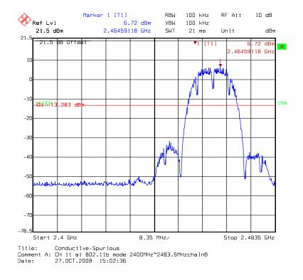
Chain B: conducted spurious @ 802.11b mode channel 11 (3 of 3)
