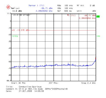
Chain B: conducted spurious @ 802.11b mode channel 6 (2 of 3)
