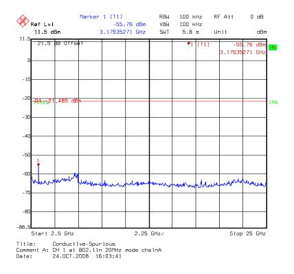
Chain A: conducted spurious @ 802.11n HT20 mode channel 6 (1 of 3)
