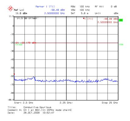
Chain C: conducted spurious @ 802.11n HT20 mode channel 6 (1 of 3)
