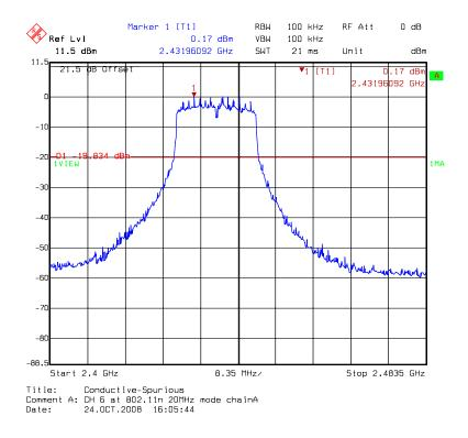
Chain A: conducted spurious @ 802.11n HT20 mode channel 6 (3 of 3)
