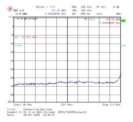
Chain C: conducted spurious @ 802.11b mode channel 11 (2 of 3)
