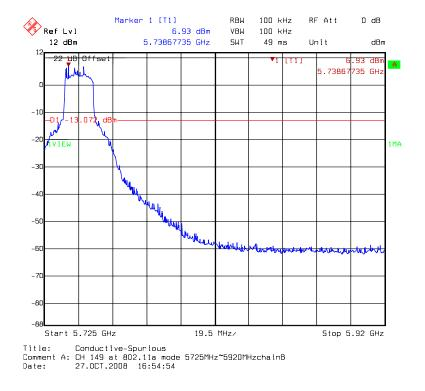
Chain B: conducted spurious @ 802.11a mode channel 149 (3 of 4)
