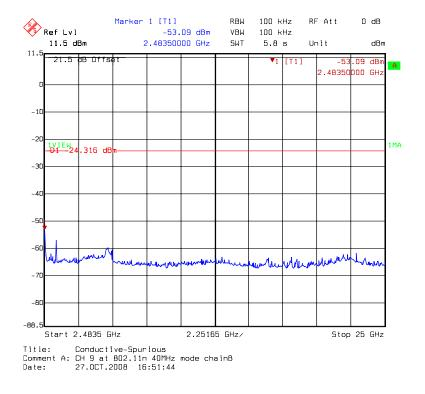
Chain B: conducted spurious @ 802.11a mode channel 149 (1 of 4)
