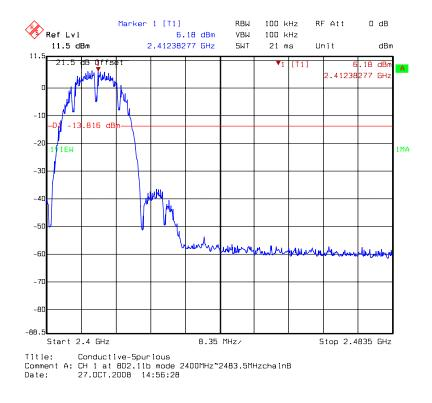
Chain B: conducted spurious @ 802.11b mode channel 1 (3 of 3)
