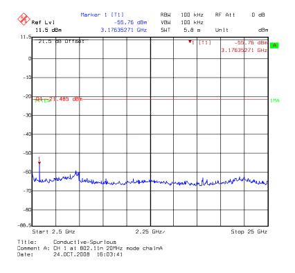
Chain A: conducted spurious @ 802.11n HT20 mode channel 157 (1 of 3)
