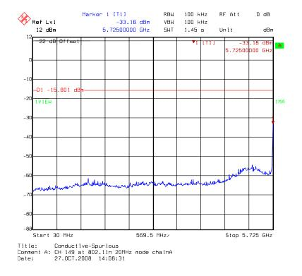
Chain A: conducted spurious @ 802.11n HT20 mode channel 149 (2 of 3)
