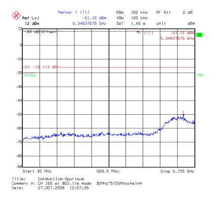
Chain A: conducted spurious @ 802.11a mode channel 165 (2 of 4)
