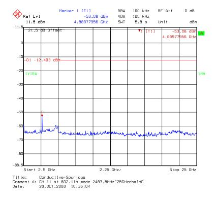
Chain C: conducted spurious @ 802.11g mode channel 1 (1 of 3)
