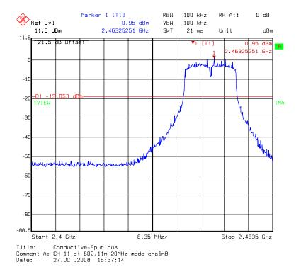
Chain B: conducted spurious @ 802.11n HT20 mode channel 11 (3 of 3)
