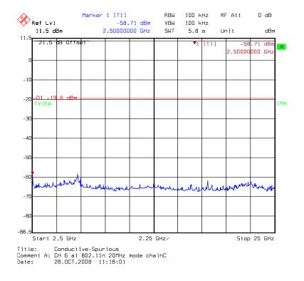
Chain C: conducted spurious @ 802.11g mode channel 11 (1 of 3)
