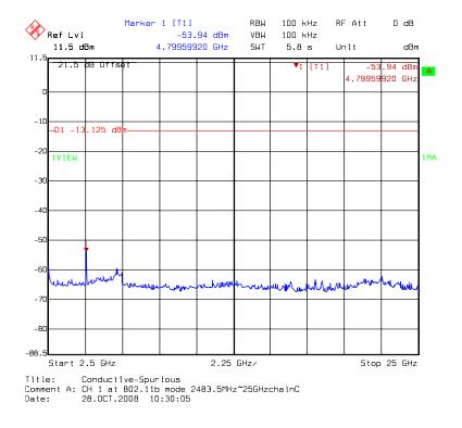
Chain C: conducted spurious @ 802.11b mode channel 6 (1 of 3)
