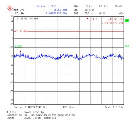
Chain C: Power Spectral Density @ 802.11n (HT20) mode channel 6
