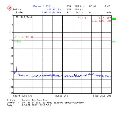
Chain A: conducted spurious @ 802.11a mode channel 165 (4 of 4)
