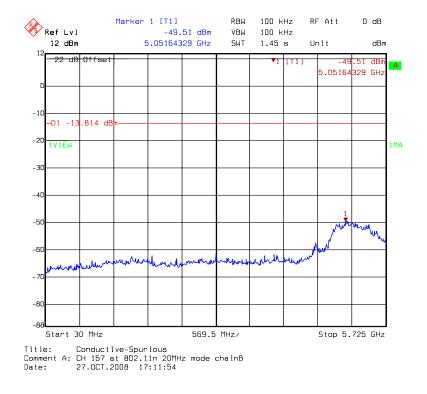
Chain B: conducted spurious @ 802.11n HT20 mode channel 157 (2 of 3)
