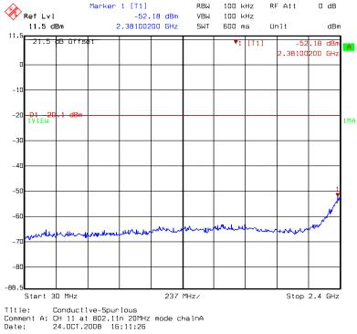
Chain A: conducted spurious @ 802.11n HT20 mode channel 11 (2 of 3)
