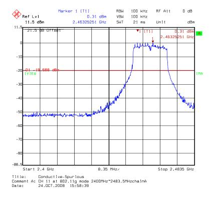
Chain A: conducted spurious @ 802.11g mode channel 11 (3 of 3)
