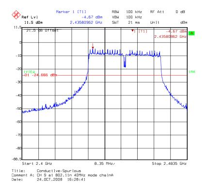
Chain A: conducted spurious @ 802.11n HT40 mode channel 9 (3 of 3)
