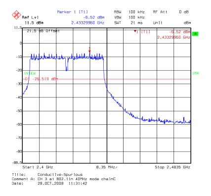
Chain C: conducted spurious @ 802.11n HT40 mode channel 3 (3 of 3)
