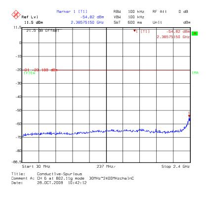
Chain C: conducted spurious @ 802.11g mode channel 6 (2 of 3)
