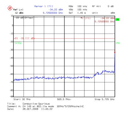
Chain C: conducted spurious @ 802.11a mode channel 149 (2 of 4)
