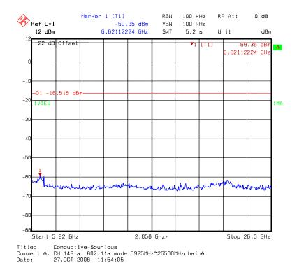
Chain A: conducted spurious @ 802.11a mode channel 149 (4 of 4)
