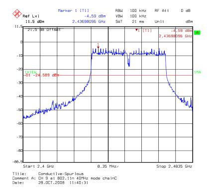
Chain C: conducted spurious @ 802.11n HT40 mode channel 9 (3 of 3)
