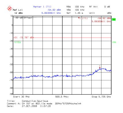
Chain A: conducted spurious @ 802.11a mode channel 157 (2 of 4)
