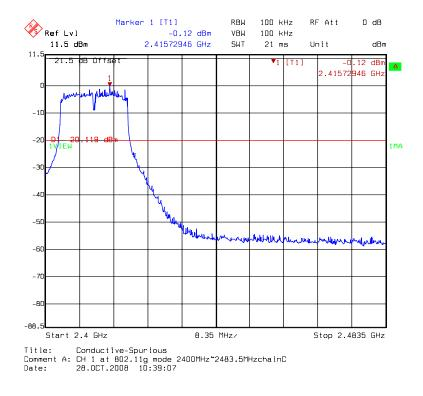
Chain C: conducted spurious @ 802.11g mode channel 1 (3 of 3)
