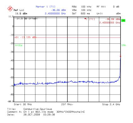
Chain C: conducted spurious @ 802.11b mode channel 1 (2 of 3)
