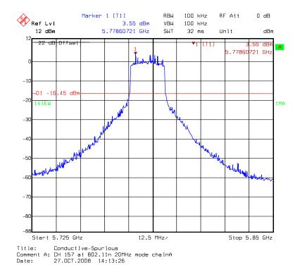
Chain A: conducted spurious @ 802.11n HT20 mode channel 157 (3 of 3)
