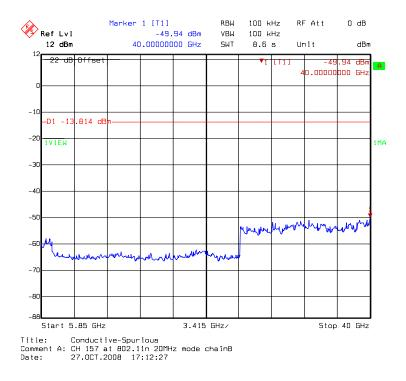
Chain B: conducted spurious @ 802.11n HT20 mode channel 165 (1 of 3)
