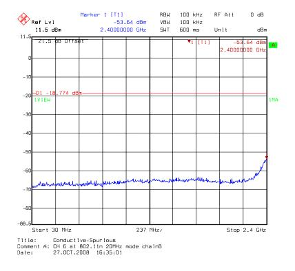
Chain B: conducted spurious @ 802.11n HT20 mode channel 6 (2 of 3)
