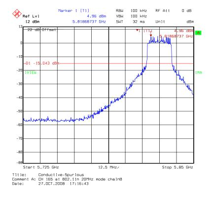
Chain B: conducted spurious @ 802.11n HT20 mode channel 165 (3 of 3)
