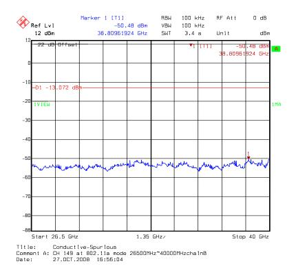
Chain B: conducted spurious @ 802.11a mode channel 157 (1 of 4)
