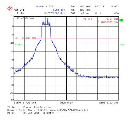
Chain B: conducted spurious @ 802.11a mode channel 157 (3 of 4)
