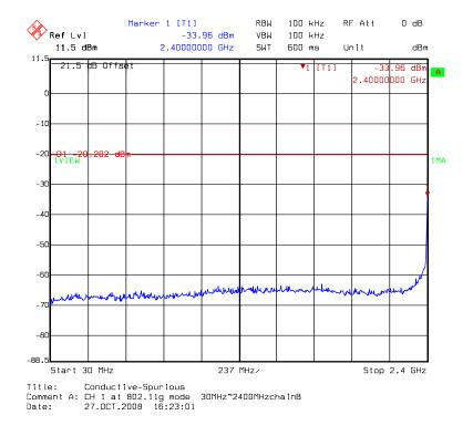
Chain B: conducted spurious @ 802.11g mode channel 1 (2 of 3)
