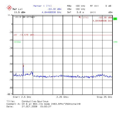
Chain B: conducted spurious @ 802.11b mode channel 11 (1 of 3)
