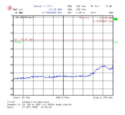
Chain A: conducted spurious @ 802.11n HT40 mode channel 159 (2 of 3)
