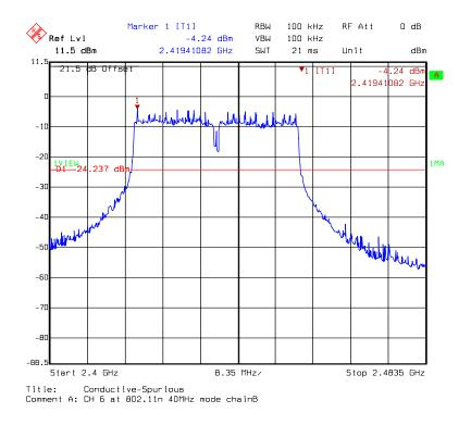
Chain B: conducted spurious @ 802.11n HT40 mode channel 6 (3 of 3)
