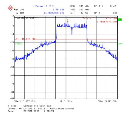
Chain B: conducted spurious @ 802.11n HT40 mode channel 159 (3 of 3)
