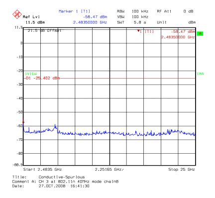
Chain B: conducted spurious @ 802.11n HT40 mode channel 6 (1 of 3)
