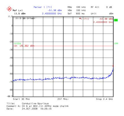
Chain A: conducted spurious @ 802.11n HT40 mode channel 6 (2 of 3)
