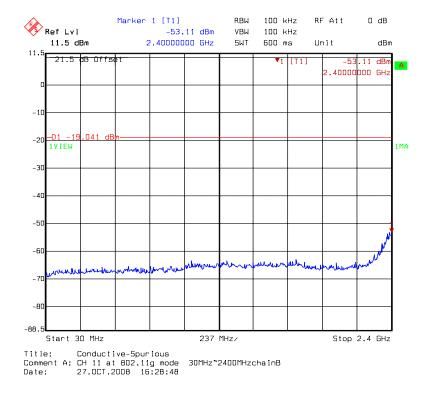
Chain B: conducted spurious @ 802.11g mode channel 11 (2 of 3)
