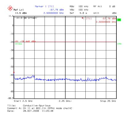
Chain C: conducted spurious @ 802.11n HT40 mode channel 3 (1 of 3)
