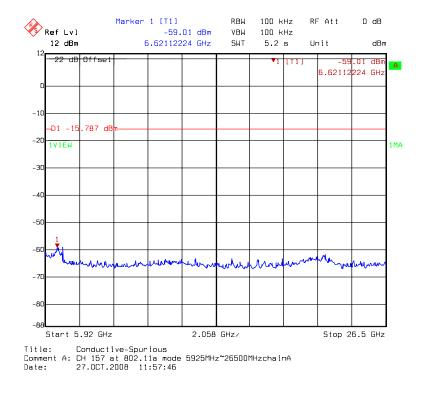
Chain A: conducted spurious @ 802.11a mode channel 157 (4 of 4)
