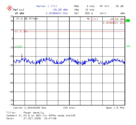
Chain B: Power Spectral Density @ 802.11n (HT40) mode channel 9
