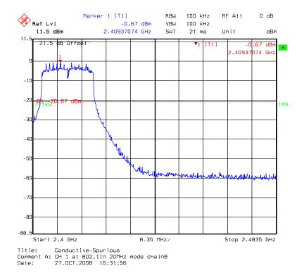
Chain B: conducted spurious @ 802.11n HT20 mode channel 1 (3 of 3)
