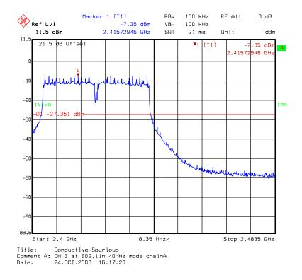
Chain A: conducted spurious @ 802.11n HT40 mode channel 3 (3 of 3)
