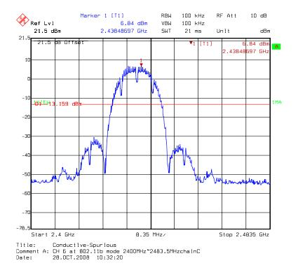
Chain C: conducted spurious @ 802.11b mode channel 6 (3 of 3)
