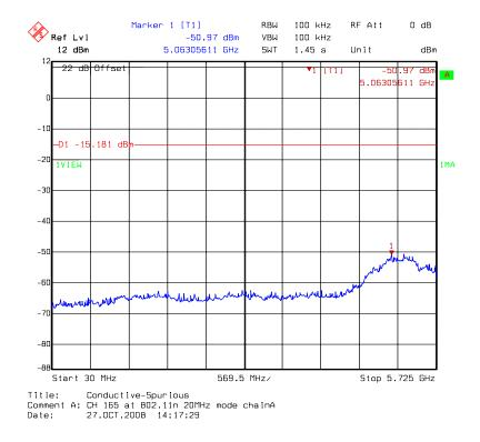
Chain A: conducted spurious @ 802.11n HT20 mode channel 165 (2 of 3)
