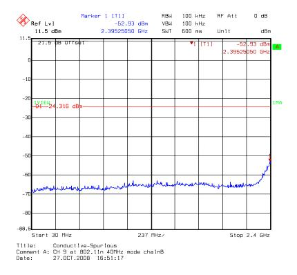
Chain B: conducted spurious @ 802.11n HT40 mode channel 9 (2 of 3)
