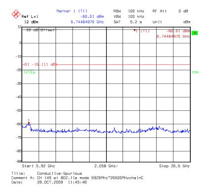
Chain C: conducted spurious @ 802.11a mode channel 149 (4 of 4)
