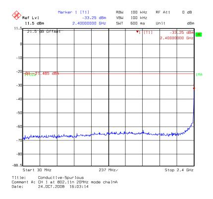
Chain A: conducted spurious @ 802.11n HT20 mode channel 1 (2 of 3)
