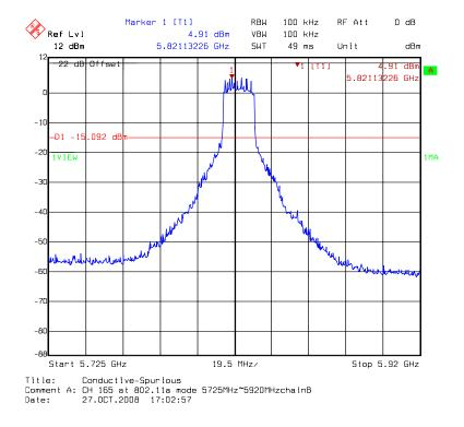
Chain B: conducted spurious @ 802.11a mode channel 165 (3 of 4)
