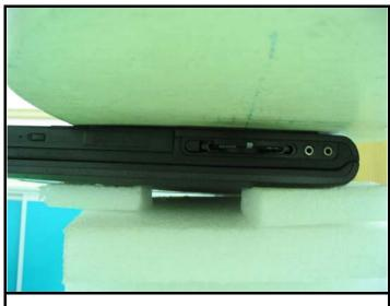
The bottom of the EUT face to the phantom with 11mm-separation distance.
