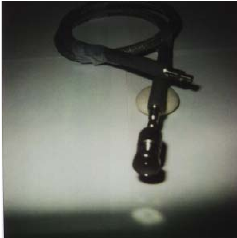
Fig. 13. Photograph of the Hewlett Packard Model 85070B Dielectric Probe. This is an open-circuited coaxial line probe.
