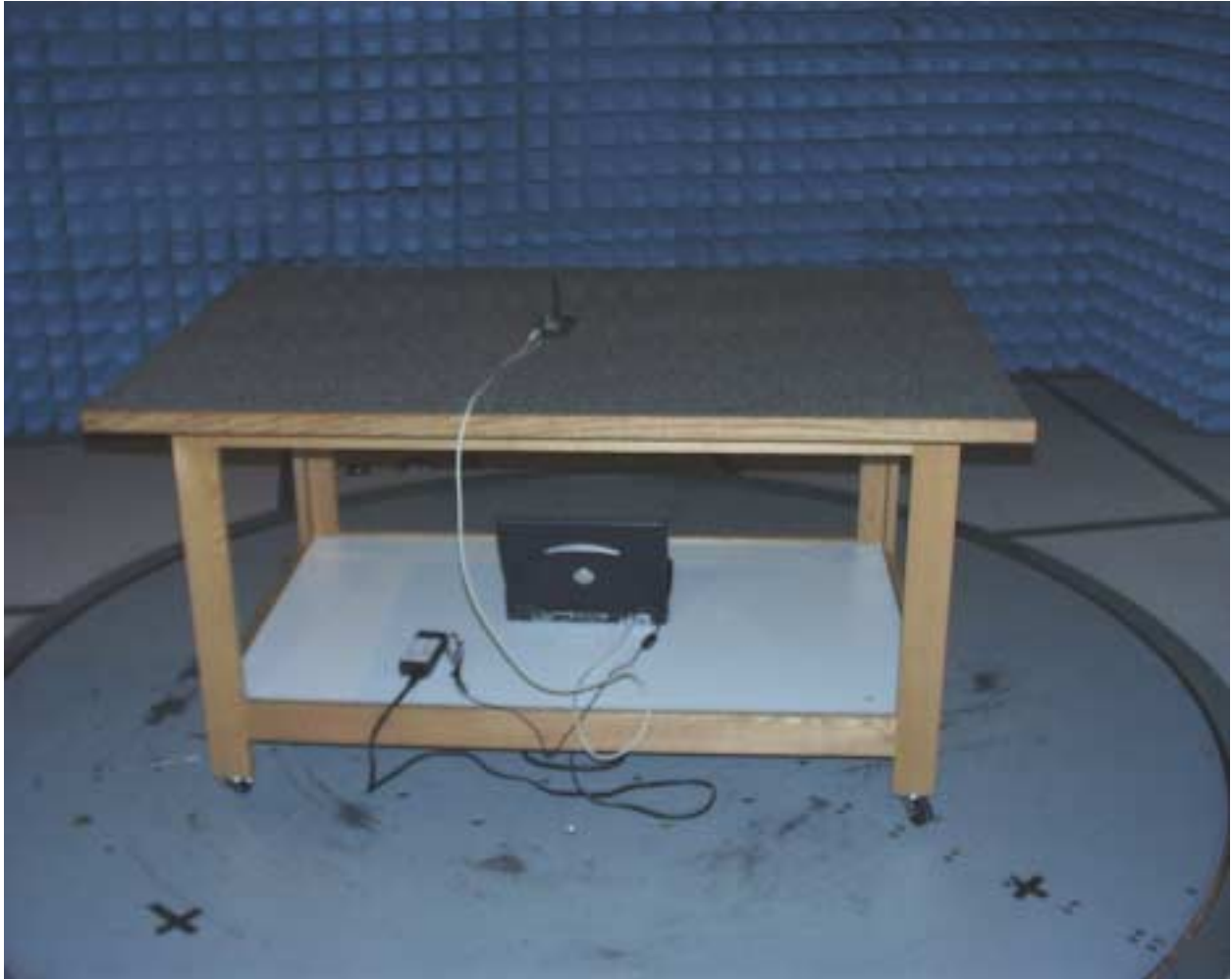
Back View Of Radiated Test Setup
