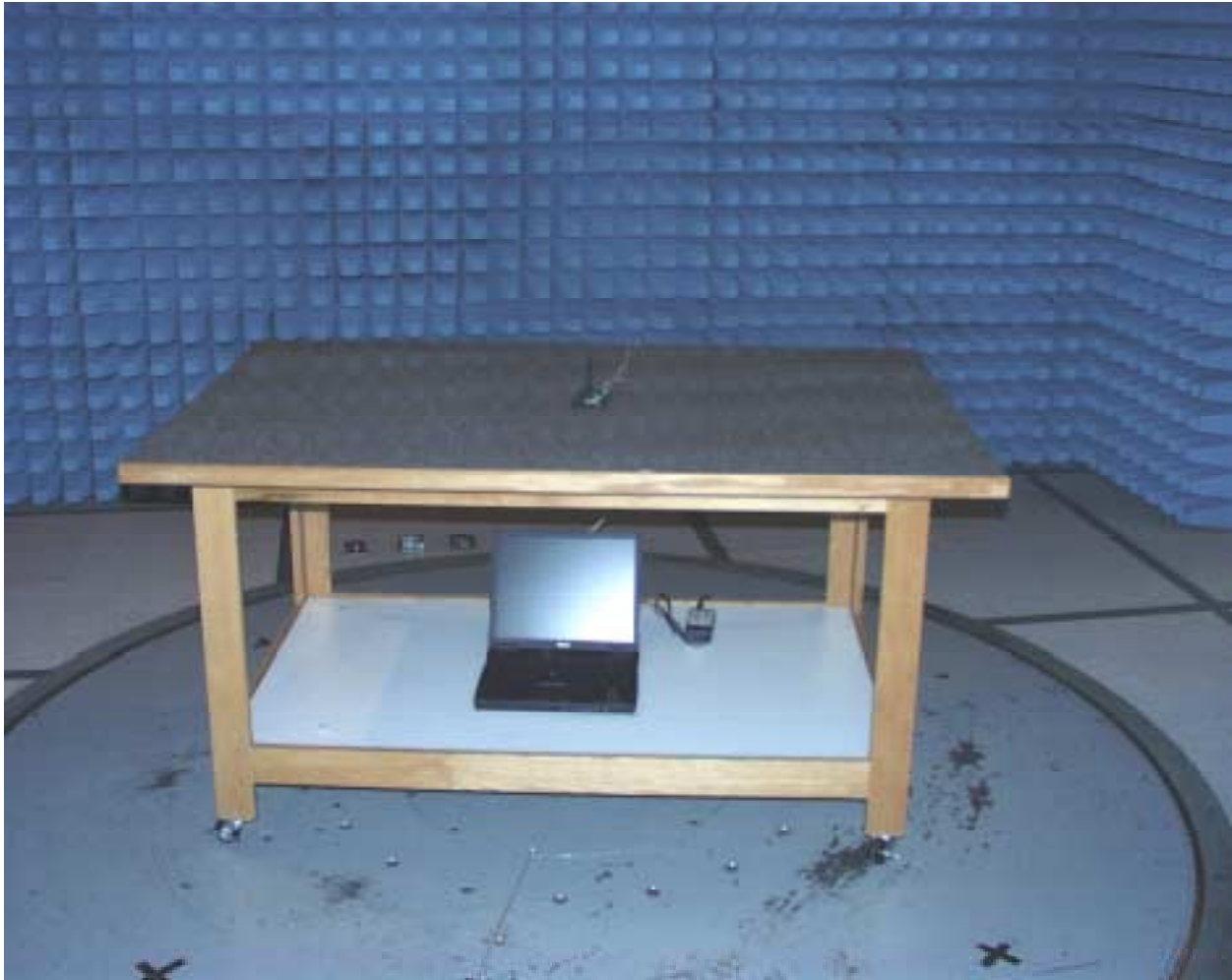
Front View of Radiated Test Setup
