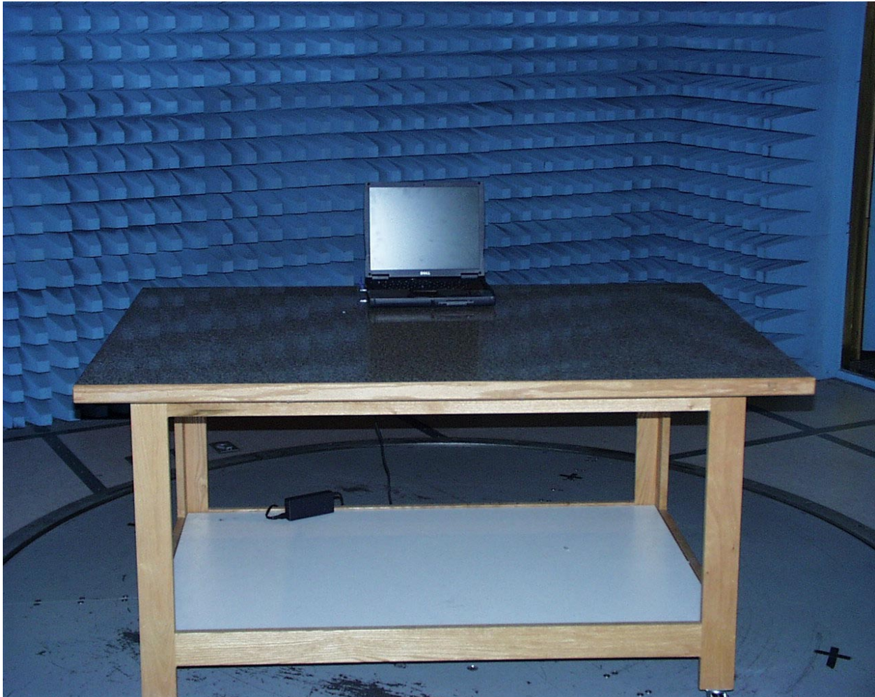
Front View of Radiated Test Setup
