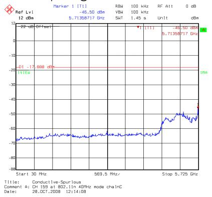
Chain C: conducted spurious @ 802.11n HT40 mode channel 159 (2 of 3)
