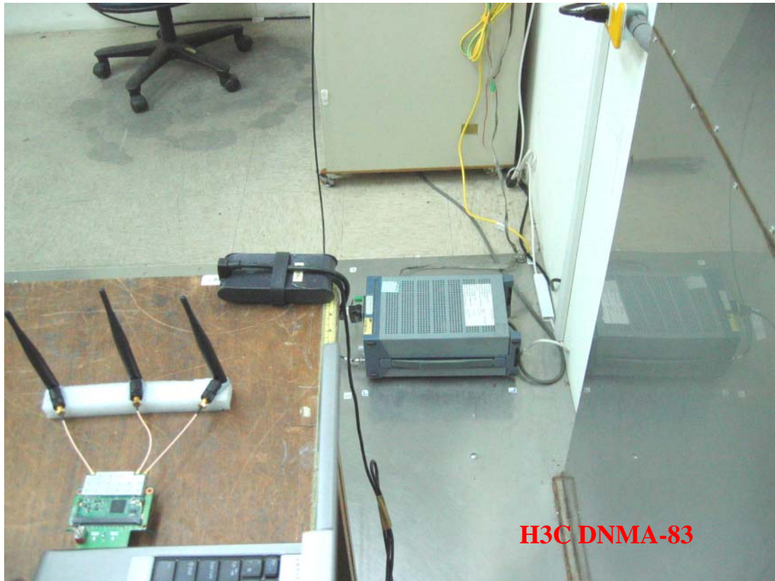
Photo 2: Conducted Emission Test Set-up photo
