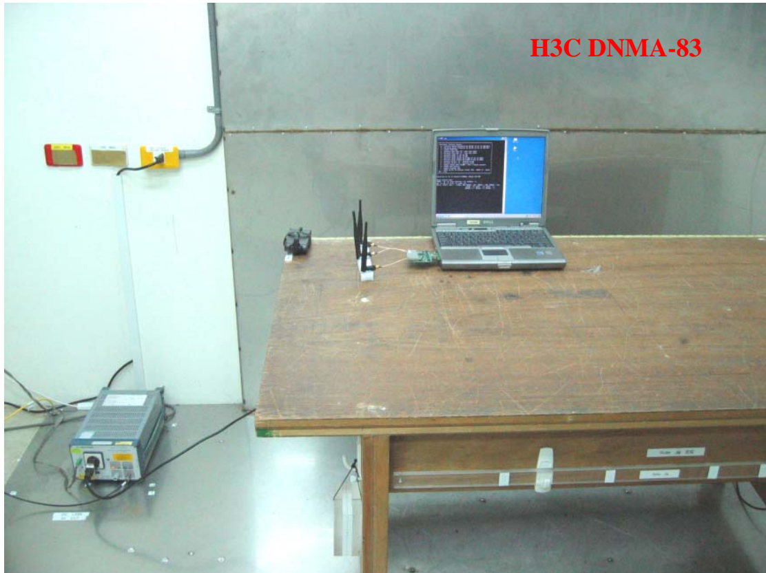
Photo 1: Conducted Emission Test Set-up photo
