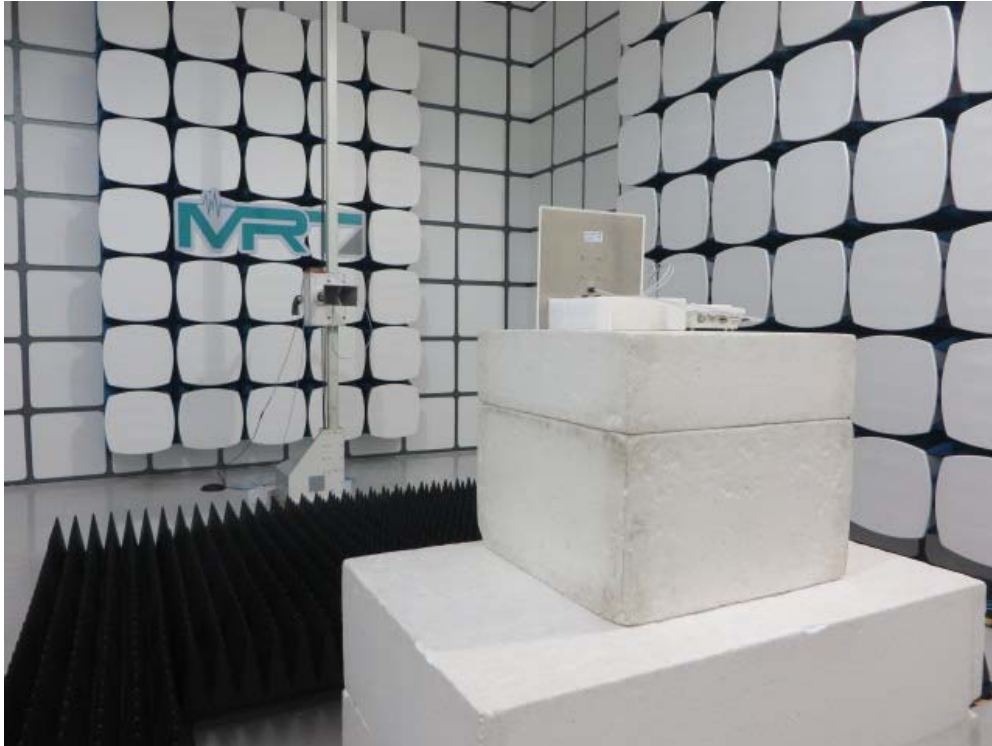
Description: Radiated Emission Test Setup for 18GHz ~ 40GHz for ANT 4#
