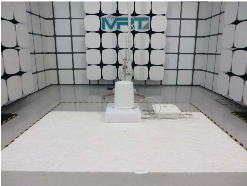
Description: Radiated Emission Test Setup for 30MHz ~ 1GHz for ANT 2#
