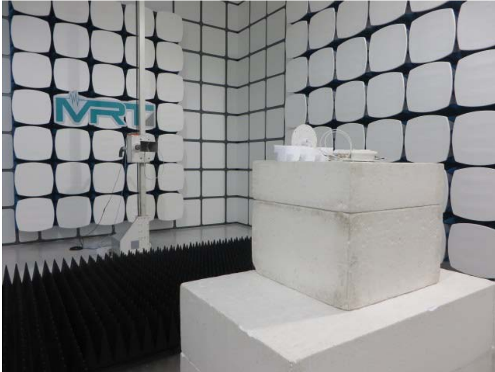
Description: Radiated Emission Test Setup for 18GHz ~ 40GHz for ANT 1#
