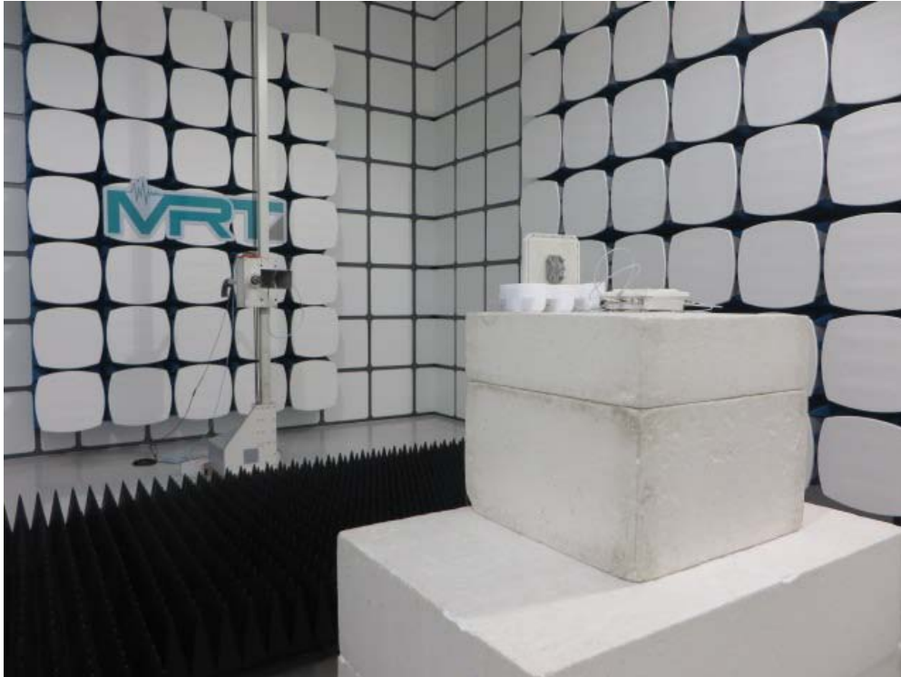
Description: Radiated Emission Test Setup for 18GHz ~ 40GHz for ANT 3#
