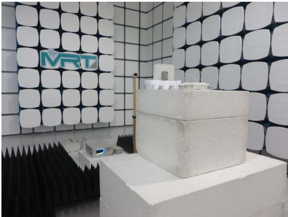
Description: Radiated Emission Test Setup for 18GHz ~ 40GHz for ANT 3#
