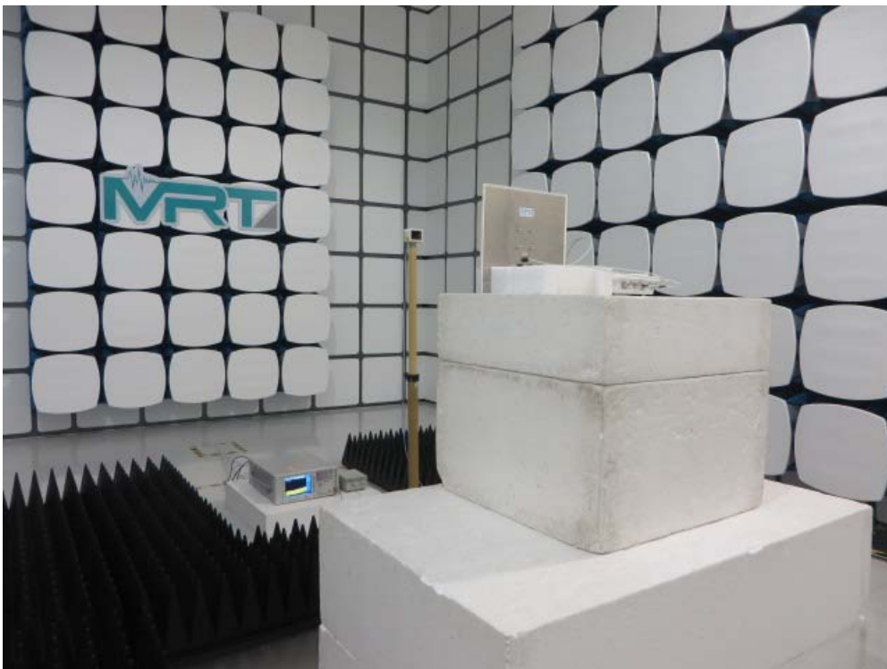
Description: Radiated Emission Test Setup for 18GHz ~ 40GHz for ANT 4#
