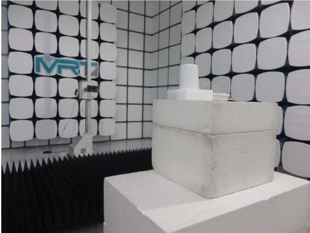
Description: Radiated Emission Test Setup for 18GHz ~ 40GHz for ANT 2#
