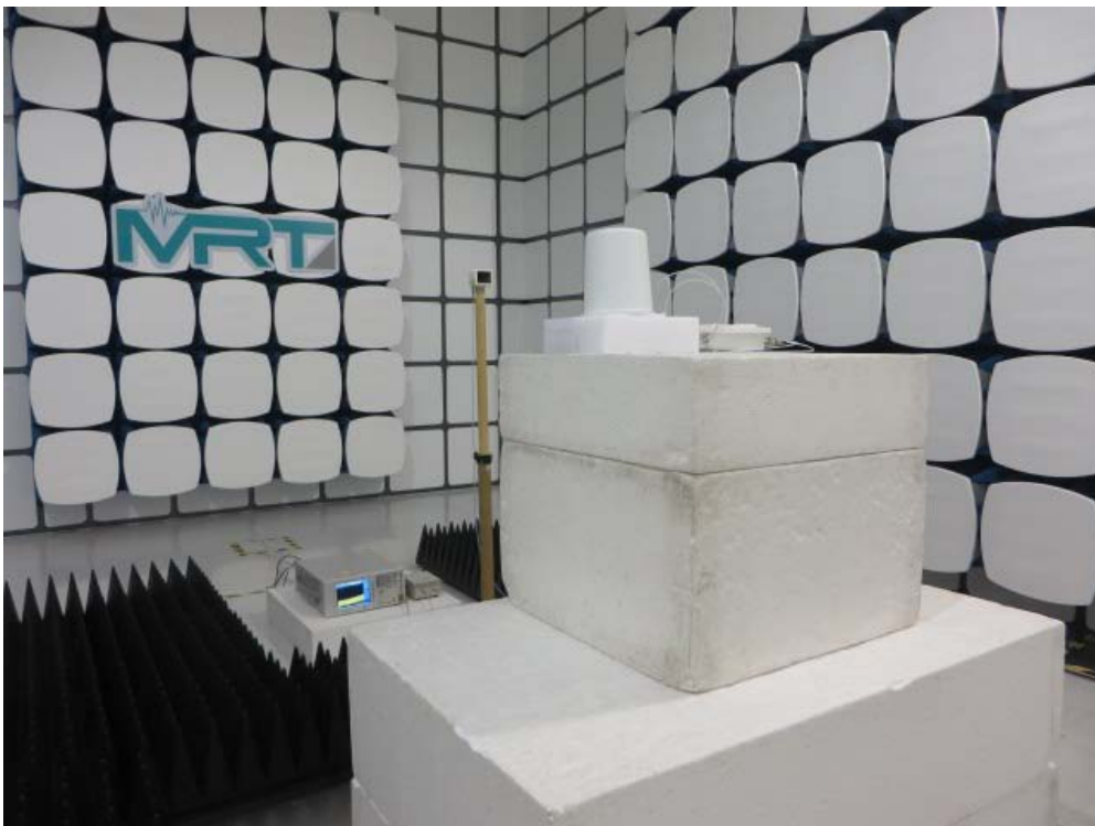
Description: Radiated Emission Test Setup for 18GHz ~ 40GHz for ANT 2#
