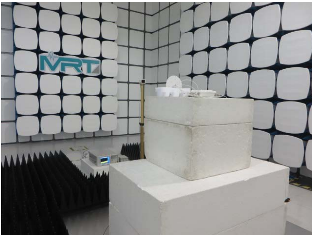
Description: Radiated Emission Test Setup for 18GHz ~ 40GHz for ANT 1#
