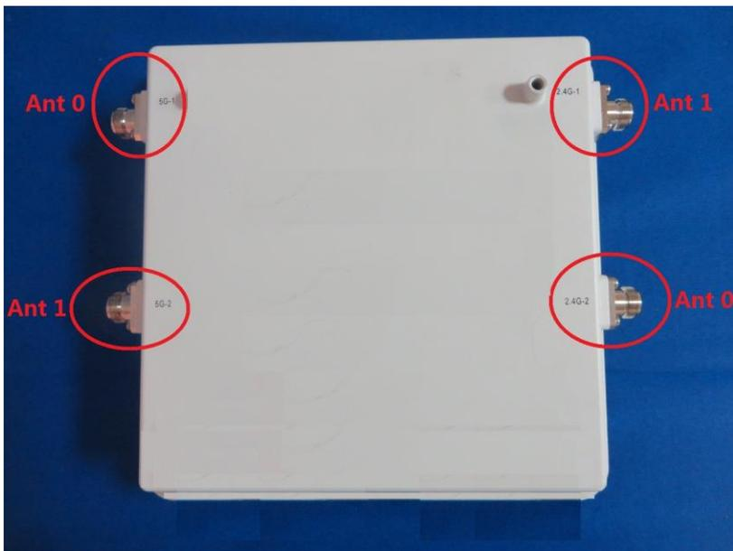
The photograph shows a white rectangular antenna module with four SMA connectors. The top-left connector is labeled '5G-1' and 'Ant 0'. The top-right connector is labeled '2.4G-1' and 'Ant 1'. The bottom-left connector is labeled '5G-2' and 'Ant 1'. The bottom-right connector is labeled '2.4G-2' and 'Ant 0'. Each connector is circled in red.
