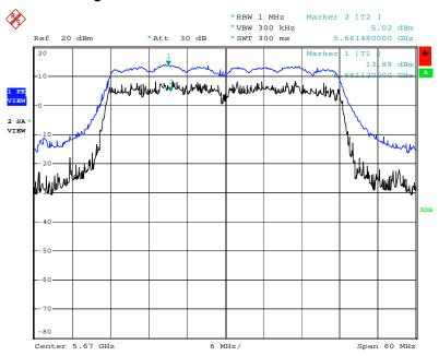
Peak Excursion Plot on Configuration Draft n MCS8 40MHz Ant. A1 + Ant. A2 + Ant. A3 / 5670 MHz
