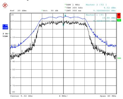
Peak Excursion Plot on Configuration Draft n MCS8 20MHz Ant. A1 + Ant. A2 + Ant. A3 / 5320 MHz
