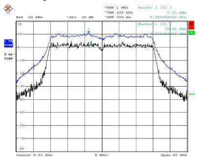
Peak Excursion Plot on Configuration Draft n MCS8 40MHz Ant. A1 + Ant. A2 + Ant. A3 / 5510MHz
