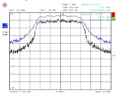
Peak Excursion Plot on Configuration Draft n MCS8 20MHz Ant. A1 + Ant. A2 + Ant. A3 / 5260 MHz
