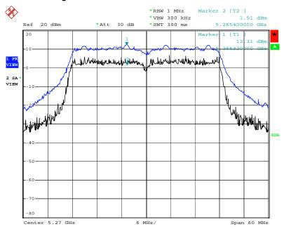
Peak Excursion Plot on Configuration Draft n MCS8 40MHz Ant. A1 + Ant. A2 + Ant. A3 / 5270 MHz
