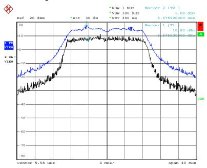
Peak Excursion Plot on Configuration Draft n MCS8 20MHz Ant. A1 + Ant. A2 + Ant. A3 / 5580 MHz
