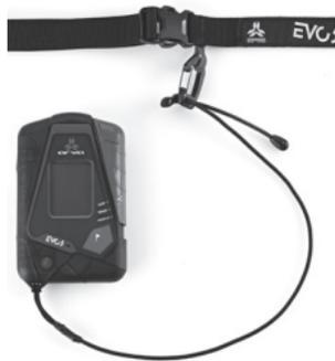
Position the EVO5 in a zippered pant pocket for the entire duration of your outing. The zipper slider should be fully closed, leaving only enough room for the elastic cord to exit. Adjust the belt around your waist and then buckle it.
