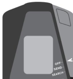
To turn on the device, push the OFF/SEND/SEARCH selector (located on the upper right-hand side of the device) down until the lock button mechanically locks it into place (the white arrow should point to "SEND").
