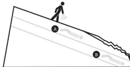
If you are not heading in the right direction, an alarm will sound and "u-turn" icon will appear on screen indicating that you should turnaround to head in the correct direction towards the victim(s) burial zone.
