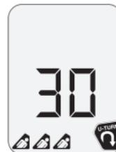
In a complex situation where there are multiple burials or in an environment where there is a lot of interference, the device might reach analysis overload. In this case, distance yourself from that specific area and then return by following another direction.
