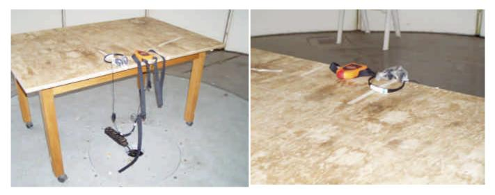
The installation of EUT is identical for pre-characterization measures in a 3 meters full anechoic chamber and for measures on a 10 meters Open site.
