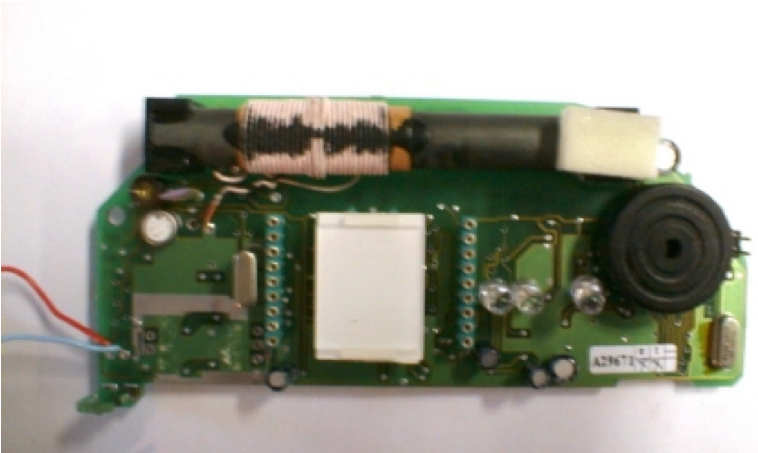
7 – Main board, display removed
