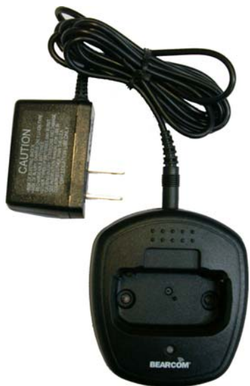
Figure 5-2) TJA-300L Charger for TJ-3100V/3400U Radio
