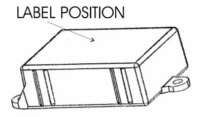
The label is (screen) printed on a plastic material, which is permanently fixed on the topside of the timing transponder.
