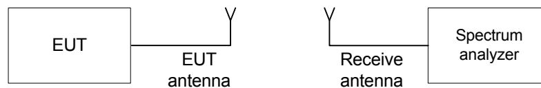
Figure 7.3.1 Occupied bandwidth test setup
