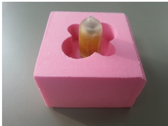
Photograph 6.4.3 EUT in Z-axis orthogonal position
