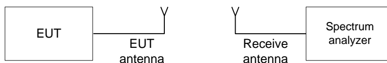
Figure 7.4.1 Occupied bandwidth test setup
