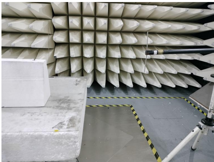
Test setup photo for measuring radiated output power without torso simulator
