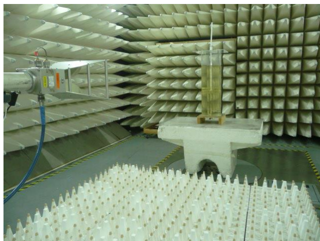
Photograph No.3 Spurious and band edge emissions measurement setup in the anechoic chamber above 1 GHz
