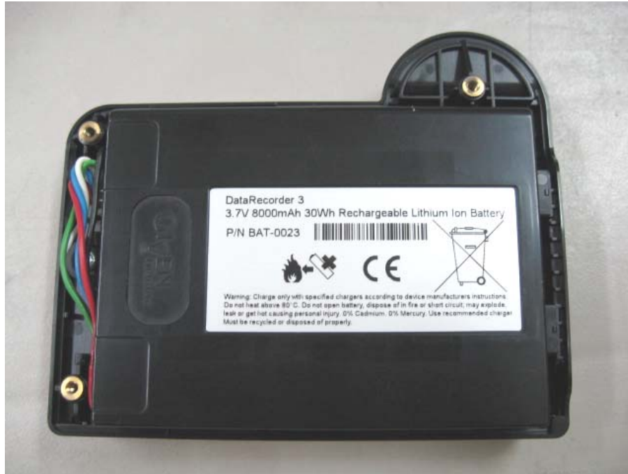
Photograph No. 5 Data recorder internal view, battery
