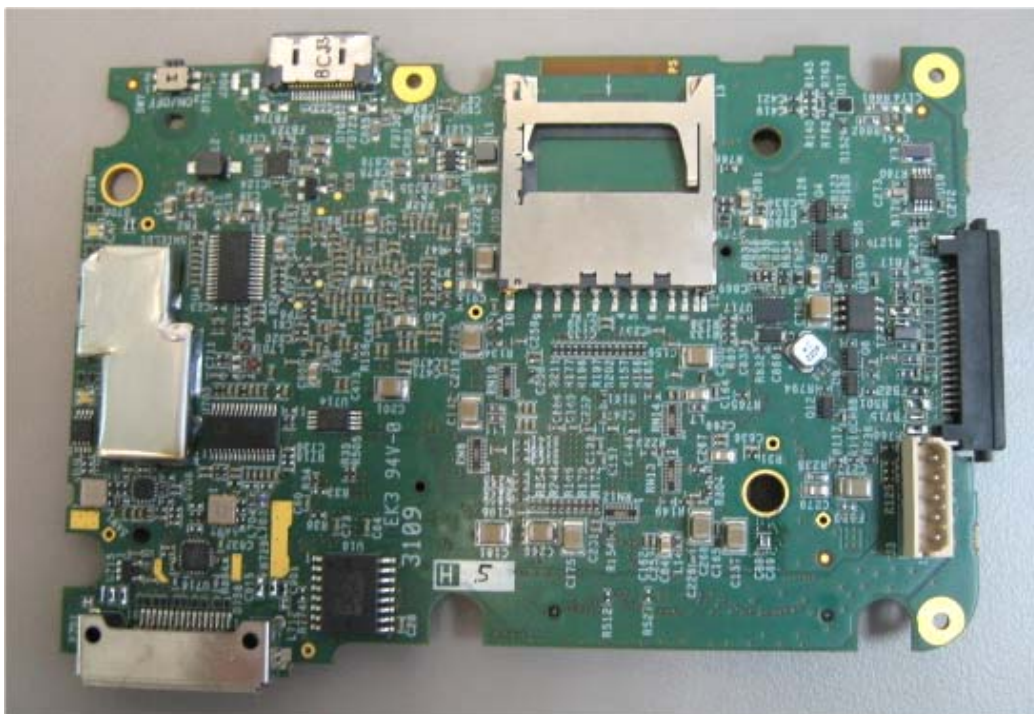
Photograph No. 3 Data recorder PCB second side view
