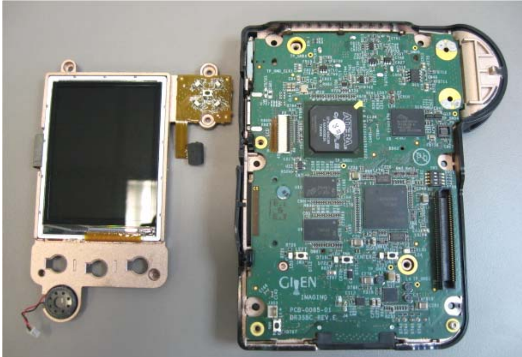
Photograph No. 2 Data recorder internal view with LCD assembly removed
