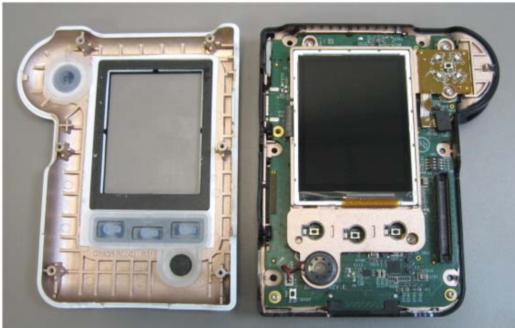
Photograph No. 1 Data recorder internal view with LCD assembly
