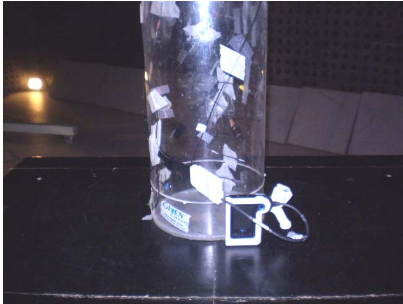
Photograph No.4 Radiated emissions measurement setup in the anechoic chamber, EUT close view
