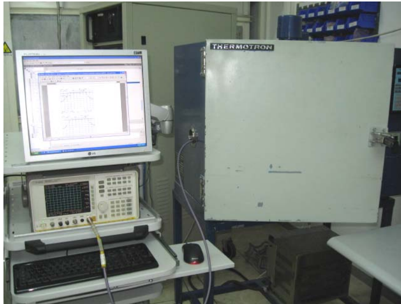
Photograph No.5 Frequency tolerance of the carrier measurement setup
