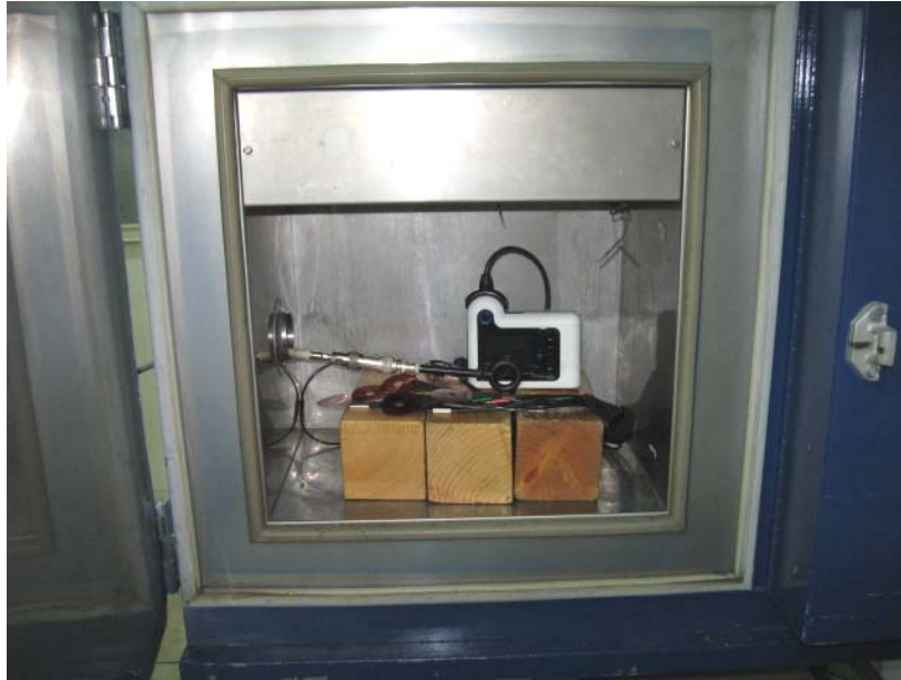
Photograph No.6 Frequency tolerance of the carrier measurement setup
