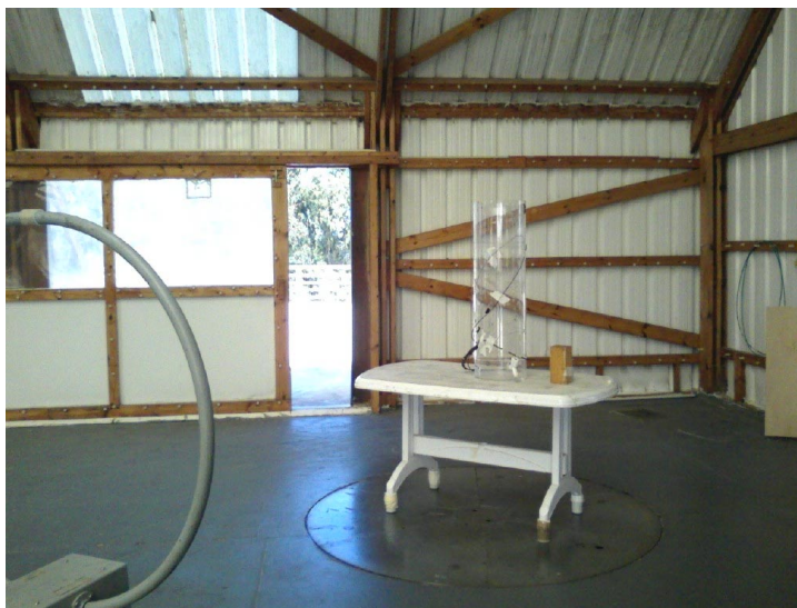
Photograph 7.1.1 Setup for in band radiated emission measurements
