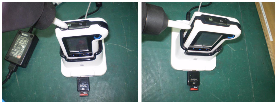
Photograph 12.1.2 Setup for immunity to ESD, EUT test points
