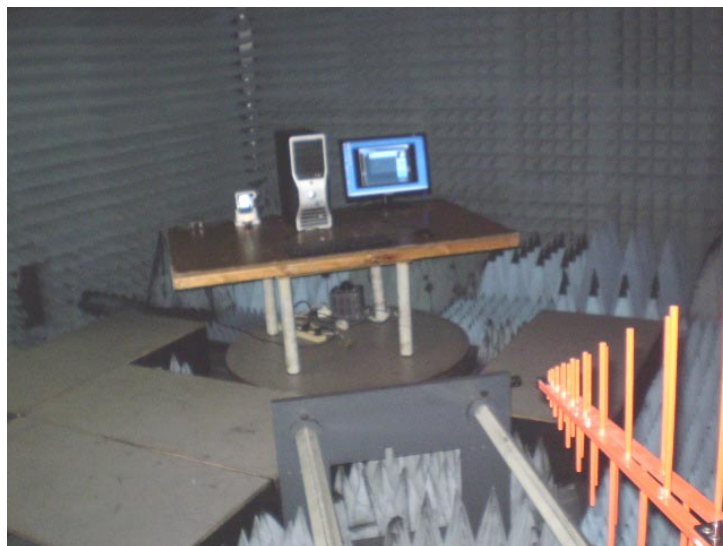
Photograph 7.2.1 Setup for preliminary radiated emission measurements below 1 GHz, general view
