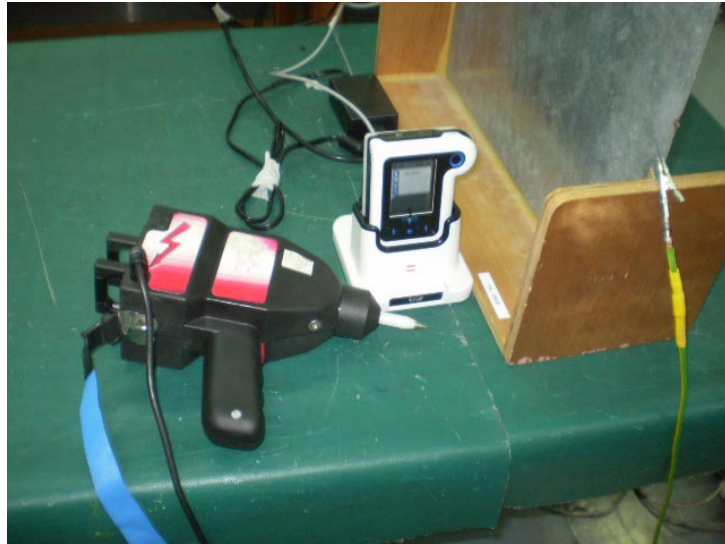
Photograph 12.1.2 Setup for immunity to ESD, EUT test points
