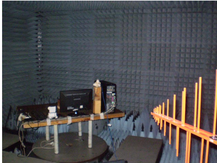
Photograph 12.2.2 Setup for radiated immunity to RF electromagnetic field test, EUT cabling
