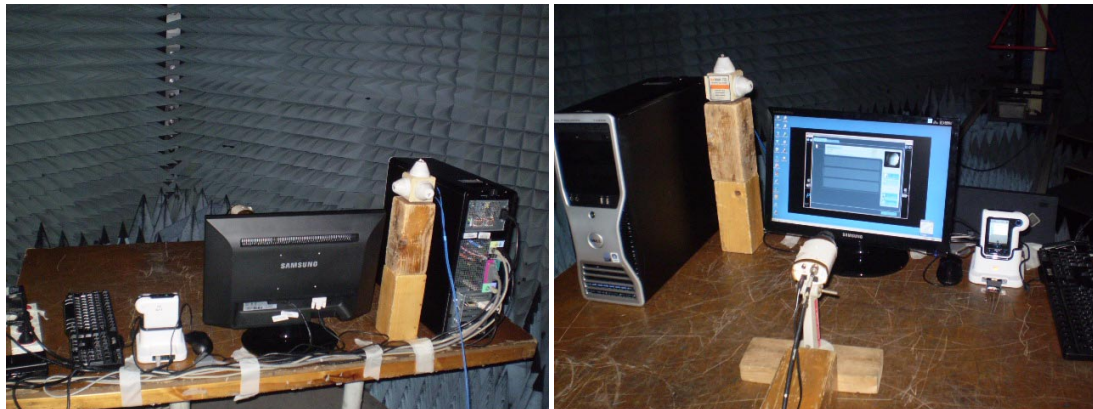
Photograph 12.2.2 Setup for radiated immunity to RF electromagnetic field test, EUT cabling
