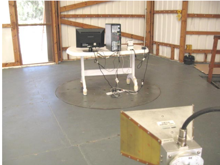
Photograph 9.2.6 Setup for final radiated disturbance measurements, EUT cabling
