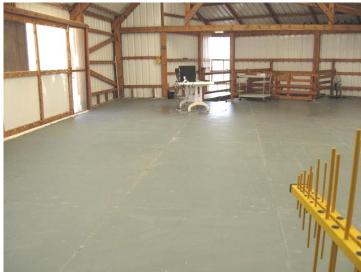
Photograph 7.2.4 Setup for final radiated emission measurements below 1 GHz, general view
