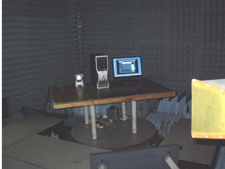
Photograph 7.2.3 Setup for preliminary radiated emission measurements, EUT cabling
