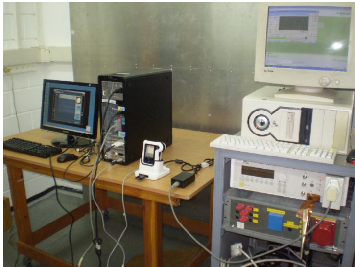
Photograph 12.4.1 Setup for conducted immunity to voltage surges at AC power line
