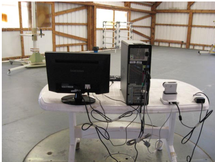
Photograph 7.2.6 Setup for final radiated emission measurements, EUT cabling
