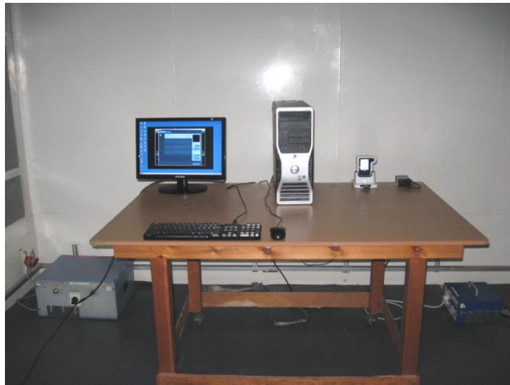
Photograph 8.1.1 Setup for conducted disturbances measurements
