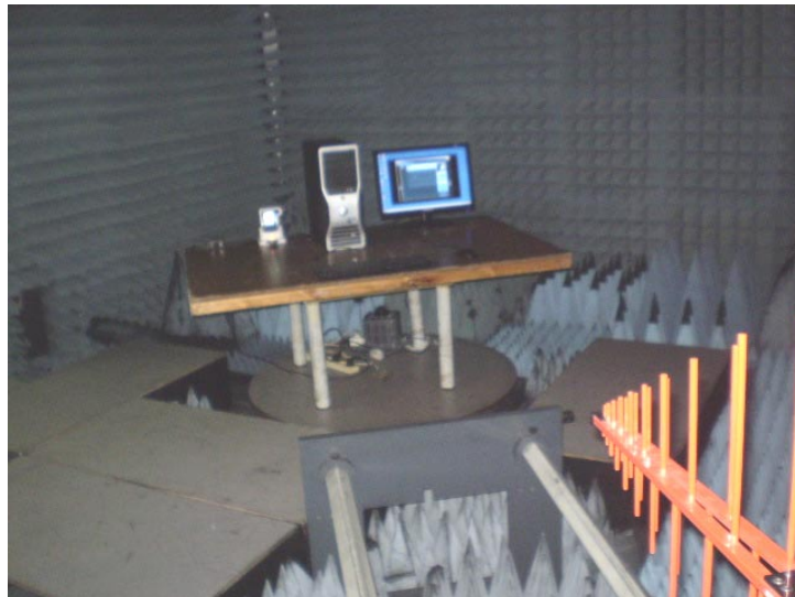
Photograph 9.2.1 Setup for preliminary radiated disturbance measurements below 1 GHz, general view
