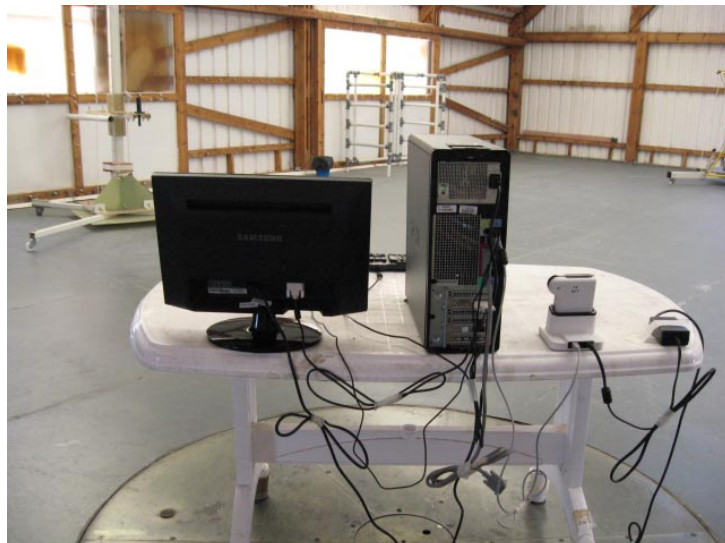
Photograph 9.2.6 Setup for final radiated disturbance measurements, EUT cabling
