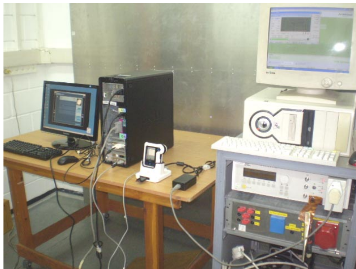
Photograph 12.7.1 Setup for immunity to voltage dips and short interruptions
