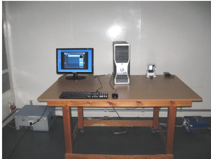
Photograph 9.1.1 Setup for conducted disturbance measurements at mains terminals
