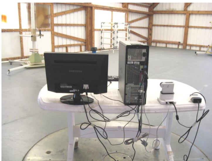
Photograph 8.2.4 Setup for final radiated disturbance measurements, EUT cabling
