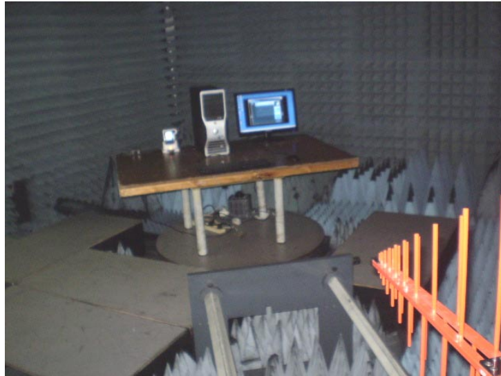
Photograph 8.2.2 Setup for preliminary radiated disturbance measurements, EUT cabling
