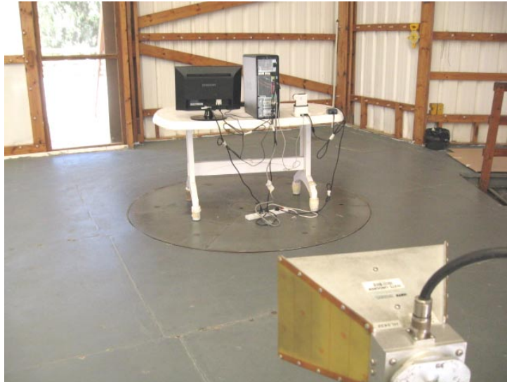
Photograph 7.2.6 Setup for final radiated emission measurements, EUT cabling
