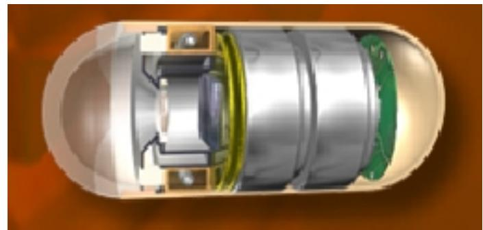
Illustration of the capsule – external view: (a) Capsule with transparent optical dome and opaque rear cover; (b) Capsule with transparent rear cover (side view show below with antenna on right-hand side); (c) Capsule with no optical dome and with no rear cover.
