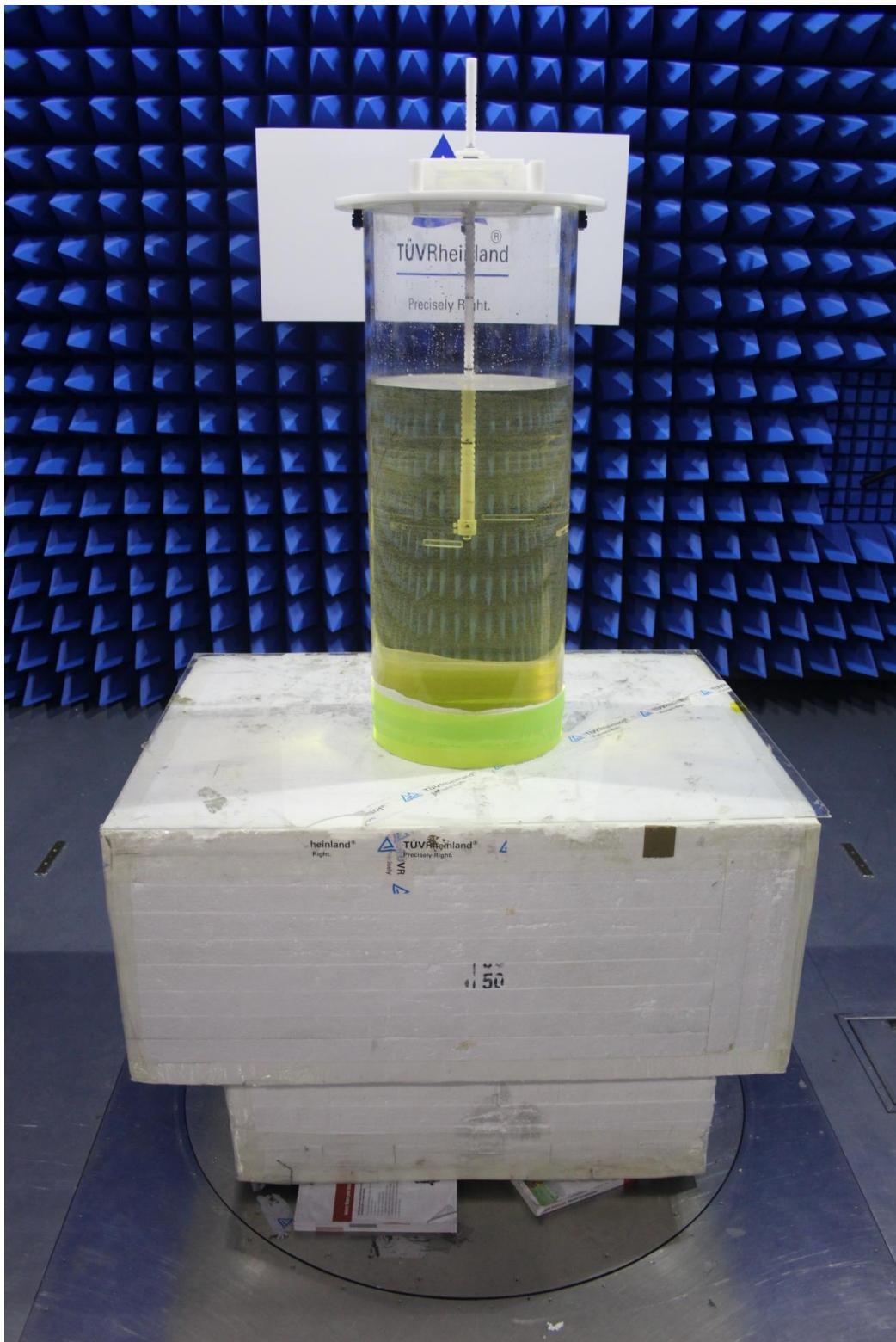
**1.1.5 Radiated emissions, testsetup arrangement views, EUT positioning, Horizontal (X) position**
