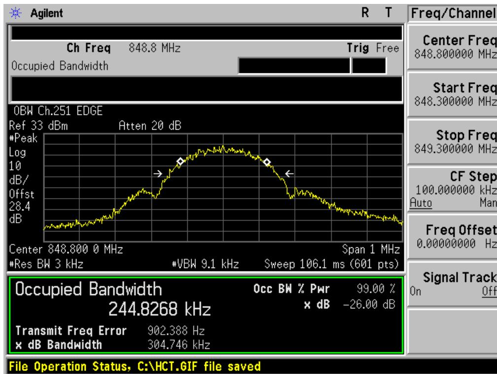
■ GSM1900 MODE (512 CH.) Occupied Bandwidth
