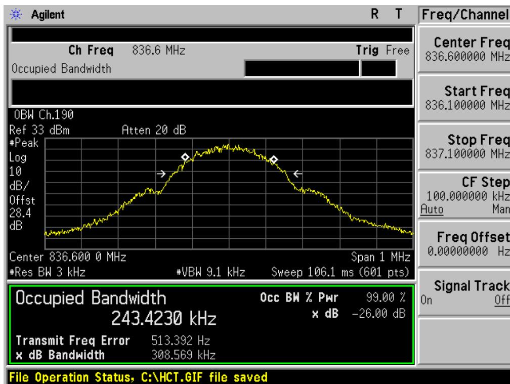
■ GSM850 MODE (251 CH.) Occupied Bandwidth
