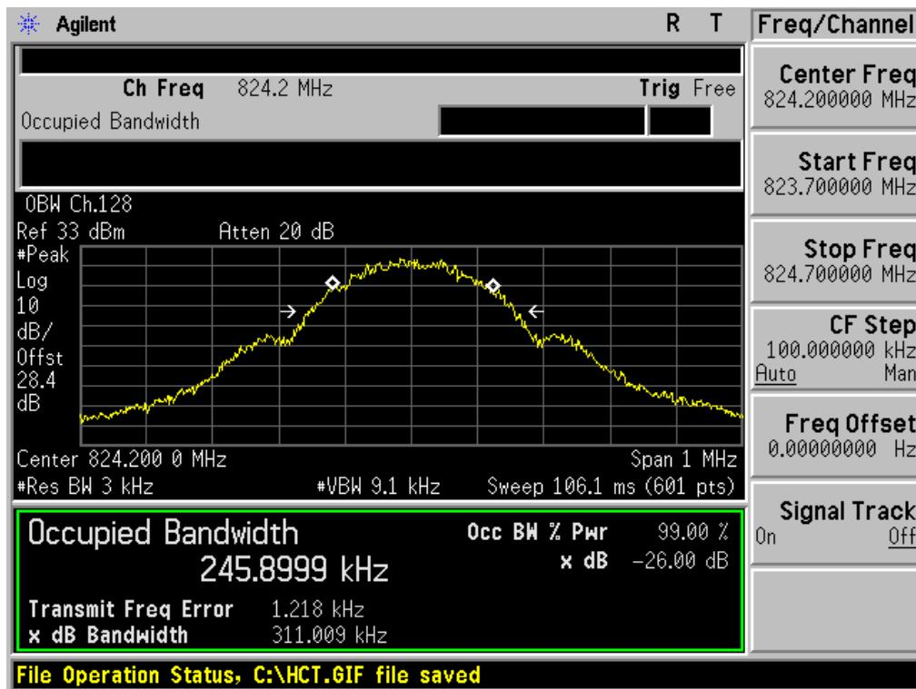
■ GSM850 MODE (190 CH.) Occupied Bandwidth
