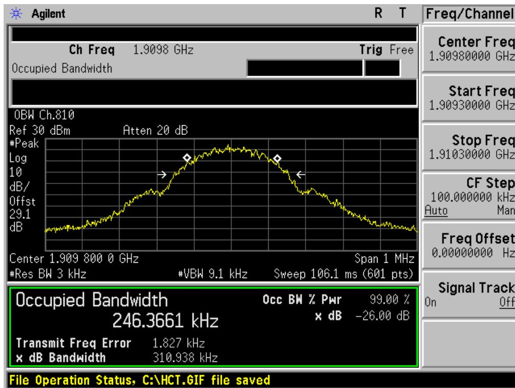
■ GSM1900 EDGE (512 CH.) Occupied Bandwidth
