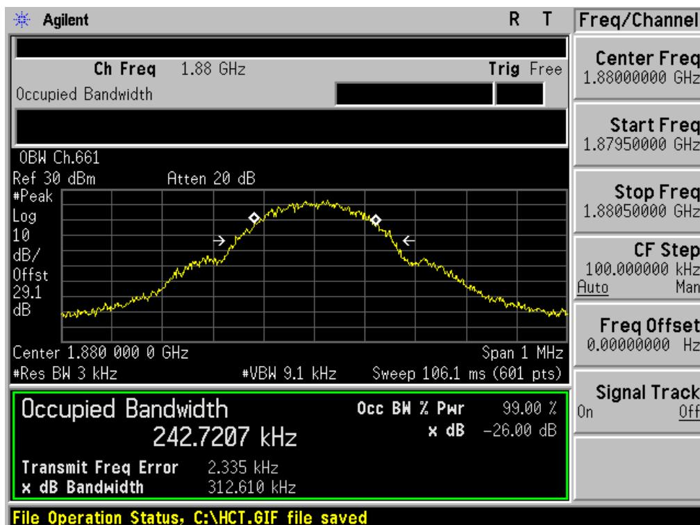
■ GSM1900 MODE (810 CH.) Occupied Bandwidth
