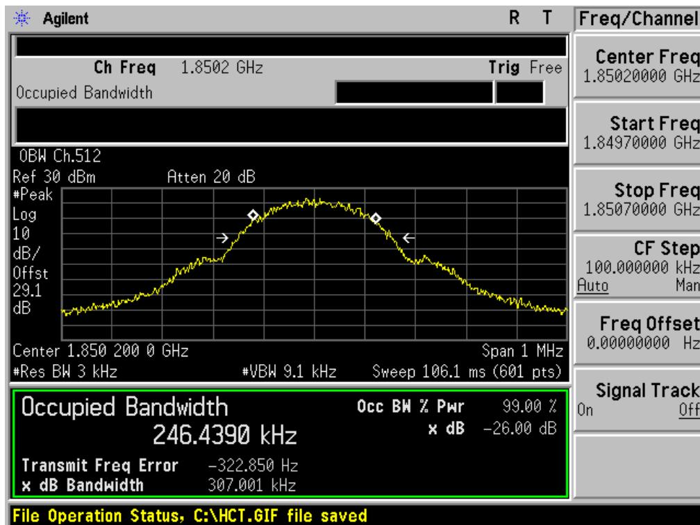
■ GSM1900 MODE (661 CH.) Occupied Bandwidth
