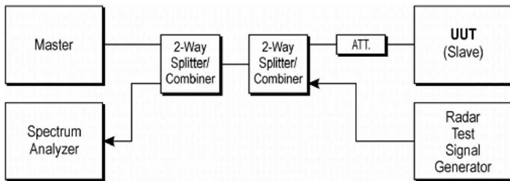
**Figure 3-1. Conducted Test Setup for DFS**
