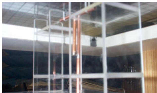
Figure 6. Validation Dipole Under Phantom
