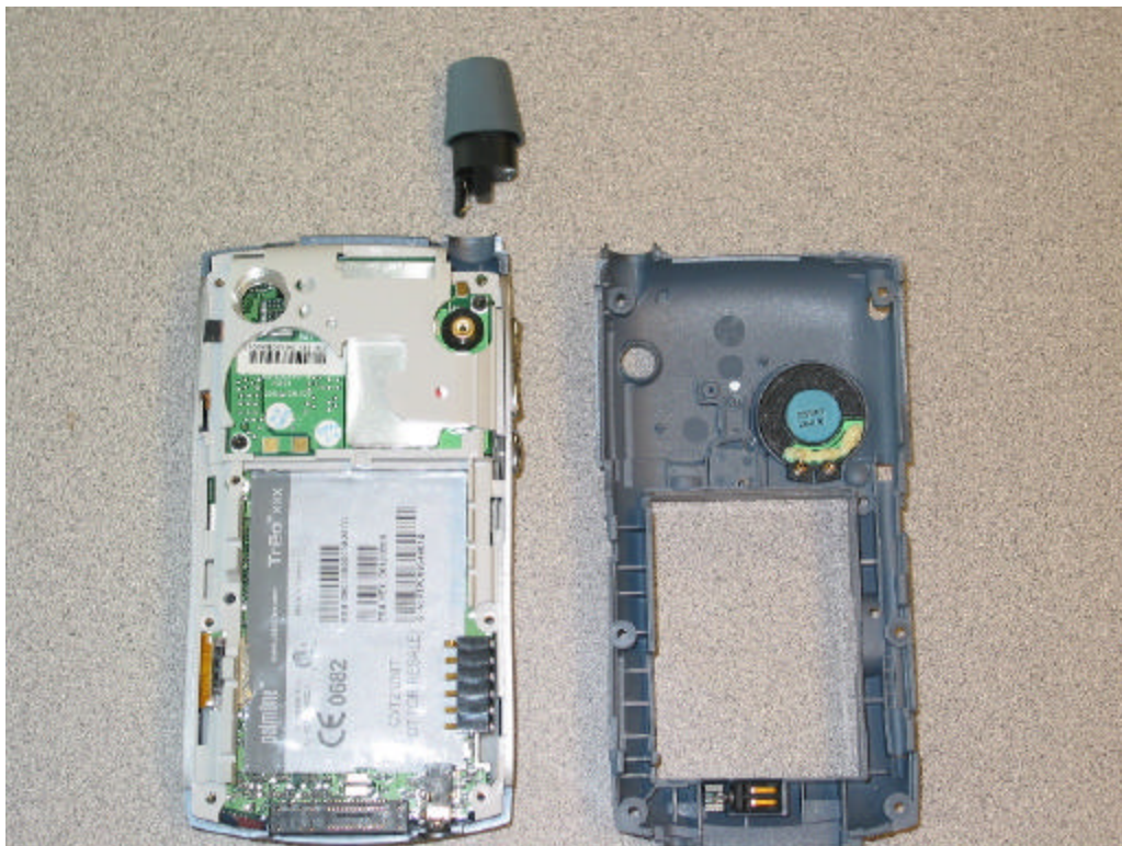
Rear cover and antenna removed
