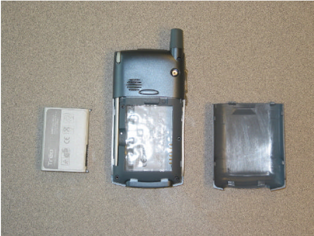
Battery and cover removed
