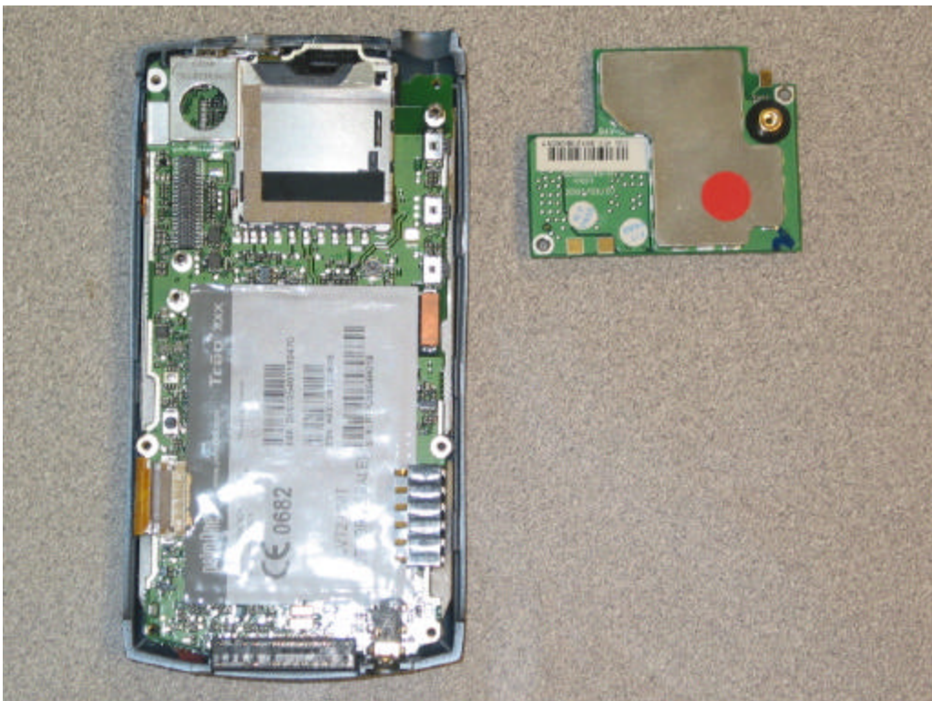
RF Module Removed
