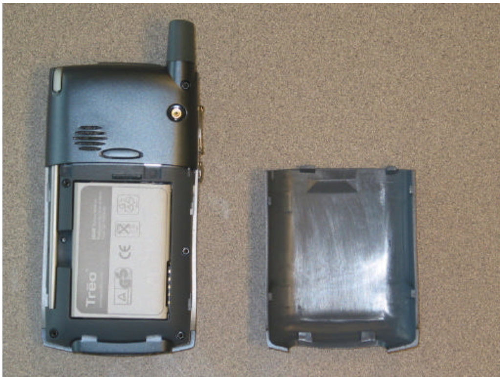
Treo 650 (CDMA) battery cover removed
