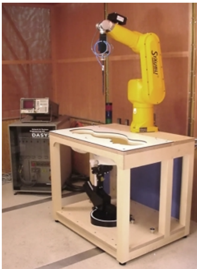
DASY3 SAR Measurement System with SAM phantom
