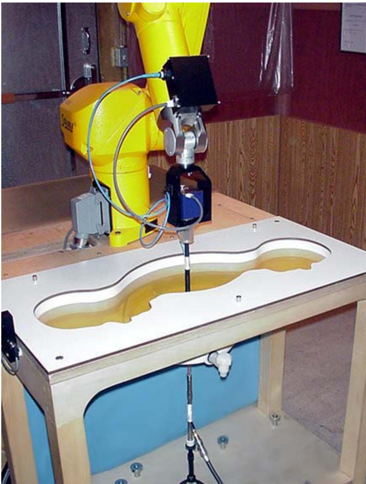
**6. 835 MHz Validation Dipole Setup**
