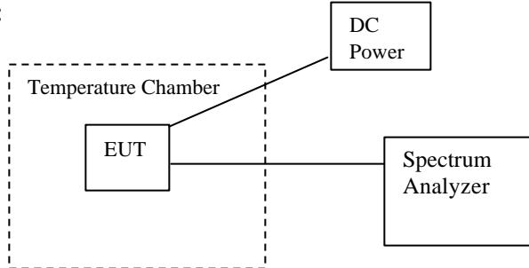
The frequency of the transmitter varied by less than 3 Hz over the temperature range of -30 to +50 degrees Celsius.
