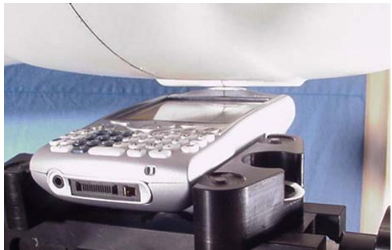
**HEAD SAR TEST SETUP PHOTOGRAPHS**
