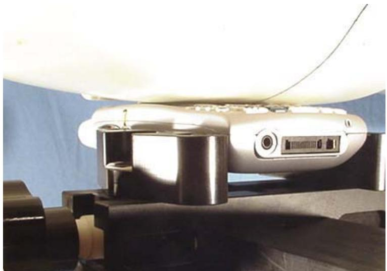
**HEAD SAR TEST SETUP PHOTOGRAPHS**
