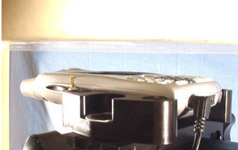
**BODY-WORN SAR TEST SETUP PHOTOGRAPHS**
