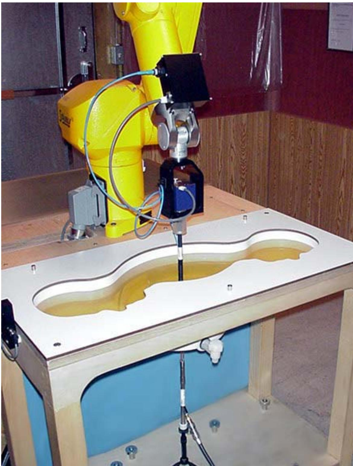
**6. 835 MHz Validation Dipole Setup**
