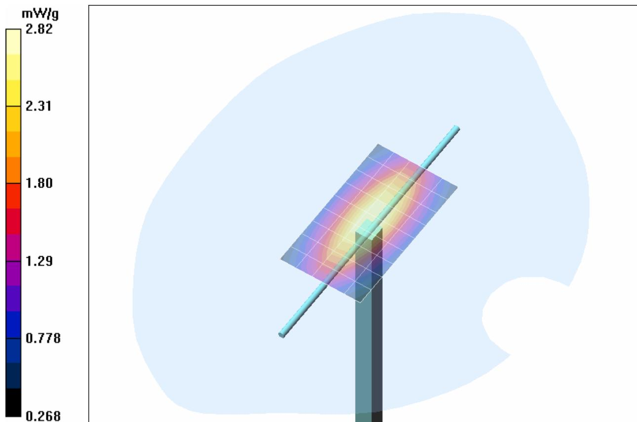
1 g average of 10 measurements: 2.60  $\text{mW/g}$
