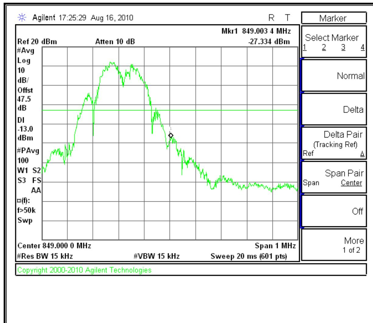
**PCS GSM1900 MODULATION RESULTS****Low Channel, Out-Of-Band Emissions**
