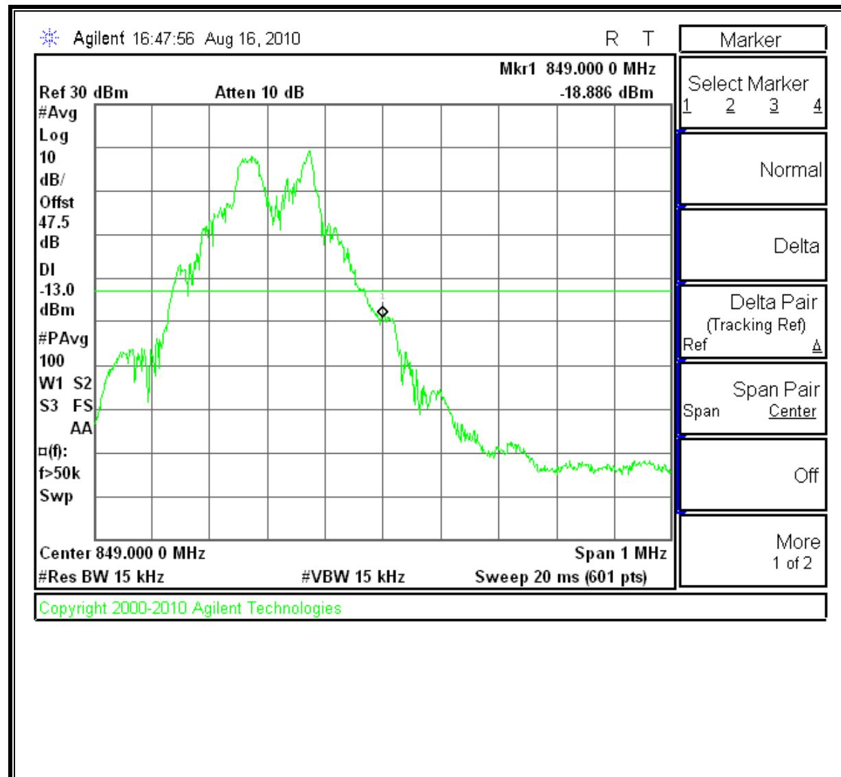
**CELL, EGPRS MODULATION:****Low Channel, Out-Of-Band Emissions**
