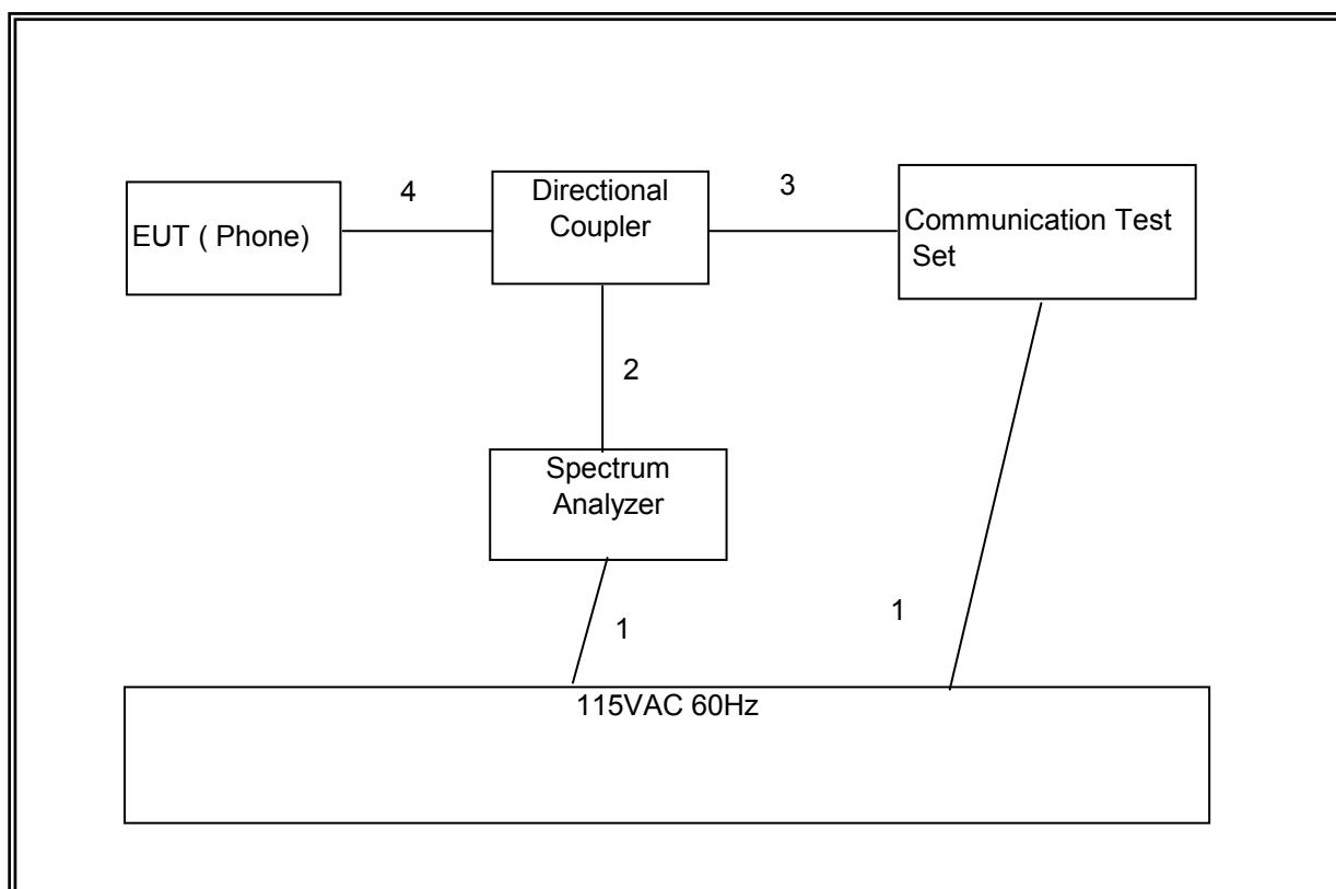
**SETUP DIAGRAM FOR RADIATED TESTS**
