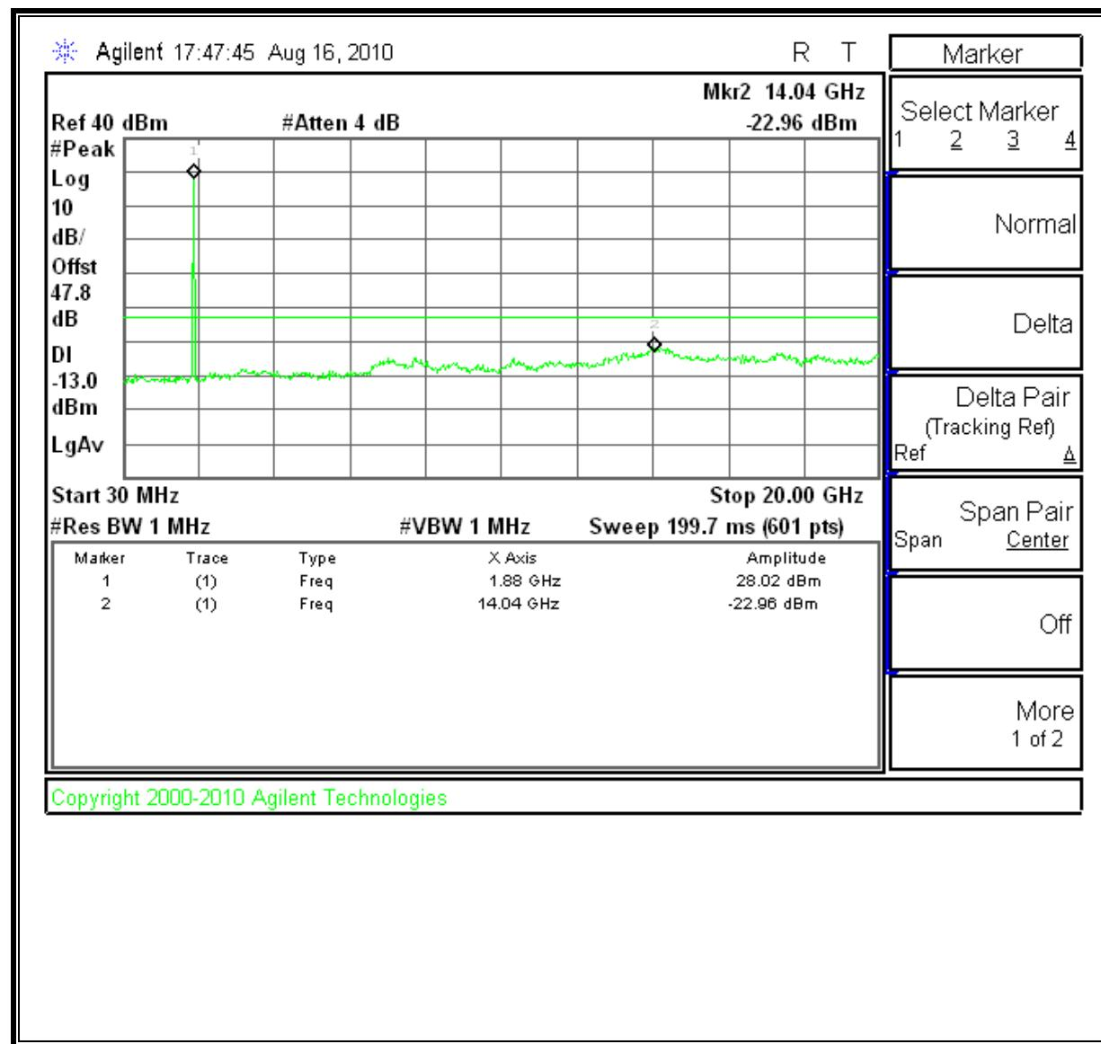
High Channel, Out-Of-Band Emissions
