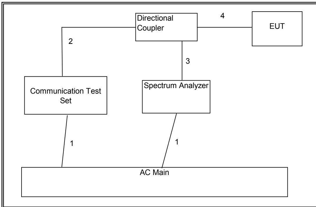
**SETUP DIAGRAM FOR RADIATED TESTS**
