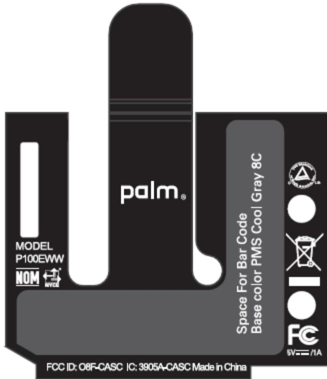
The FCC ID on your Palm phone is located on a label inside the battery compartment.
