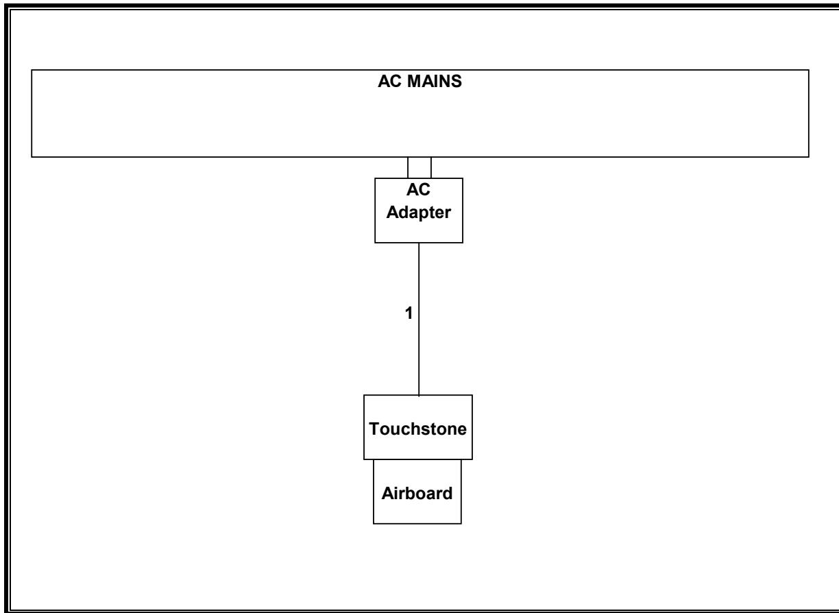
**SETUP DIAGRAM FOR TEST CONFIGURATIONS WITH DEAD BATTERY**
