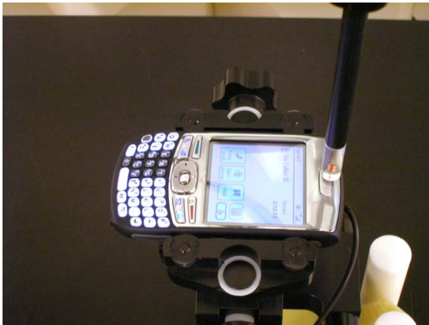
Figure 13-1 Test Setup for Wireless Device
