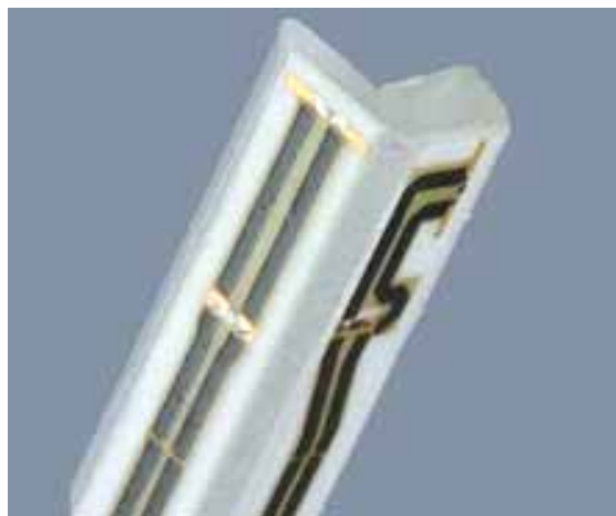
Fig. 5.2 E-field Free-space Probe
