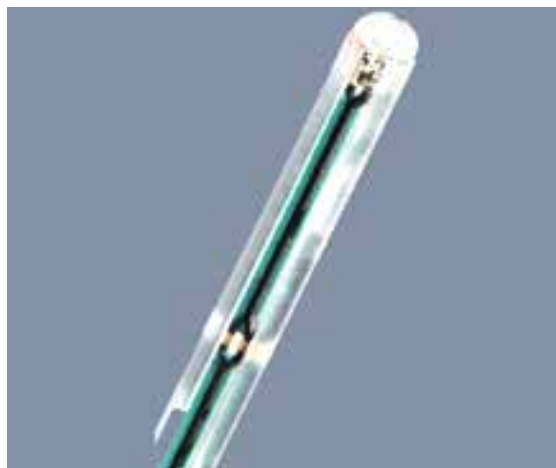
Fig. 5.3 H-field Free-space Probe
