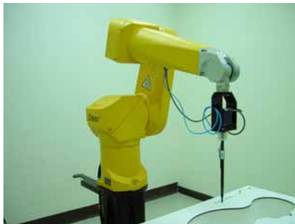
Fig. 5.2 Probe setup on robot
