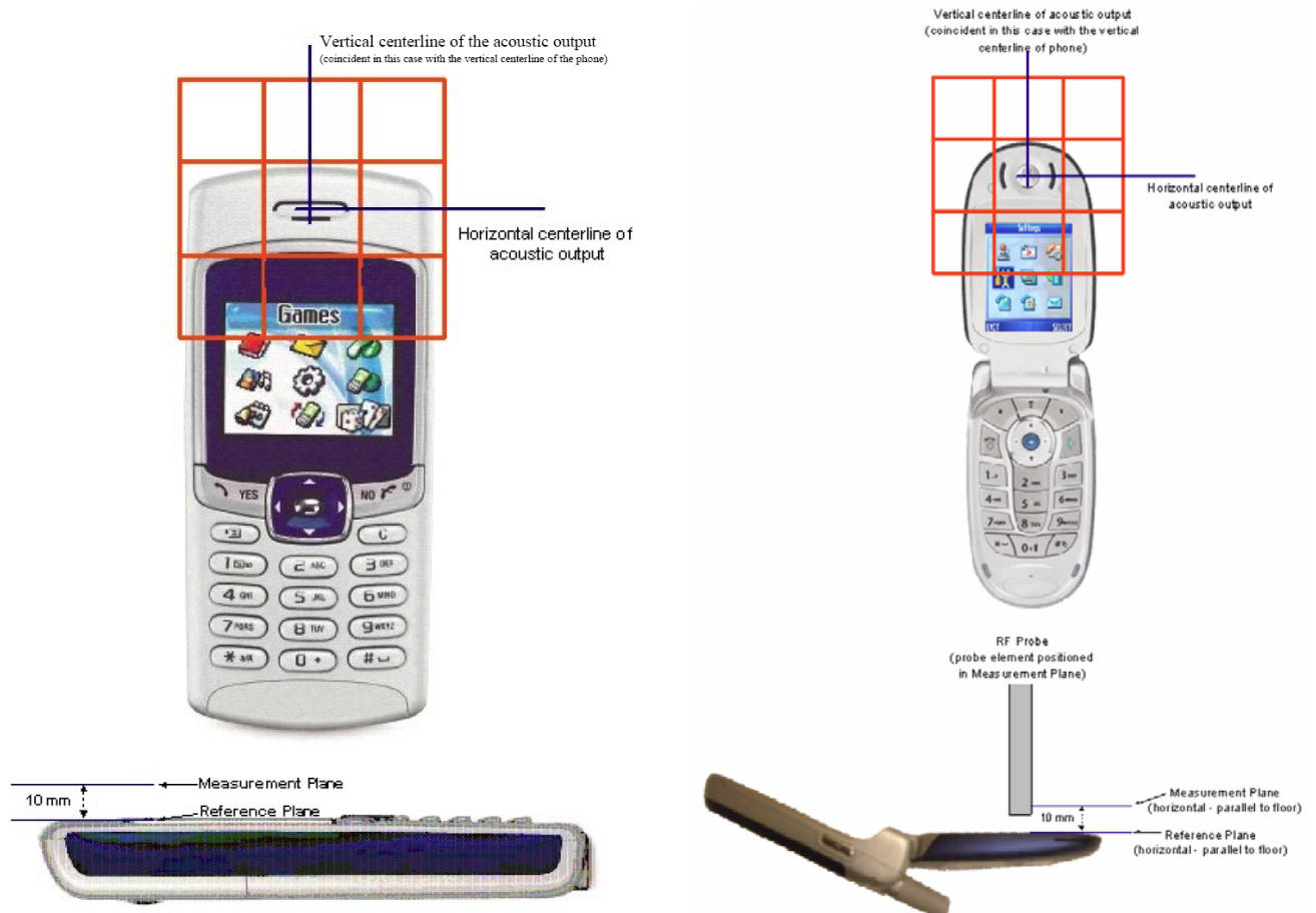
Figure 1: A typical DUT reference and plane for HAC measurements
