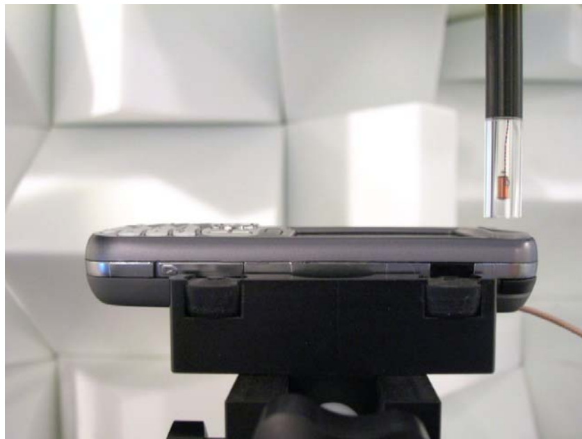
Figure 13-2 Test Setup for Wireless Device
