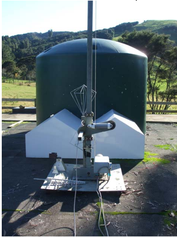
An array of antennas used at the test site on top of the antenna mast
