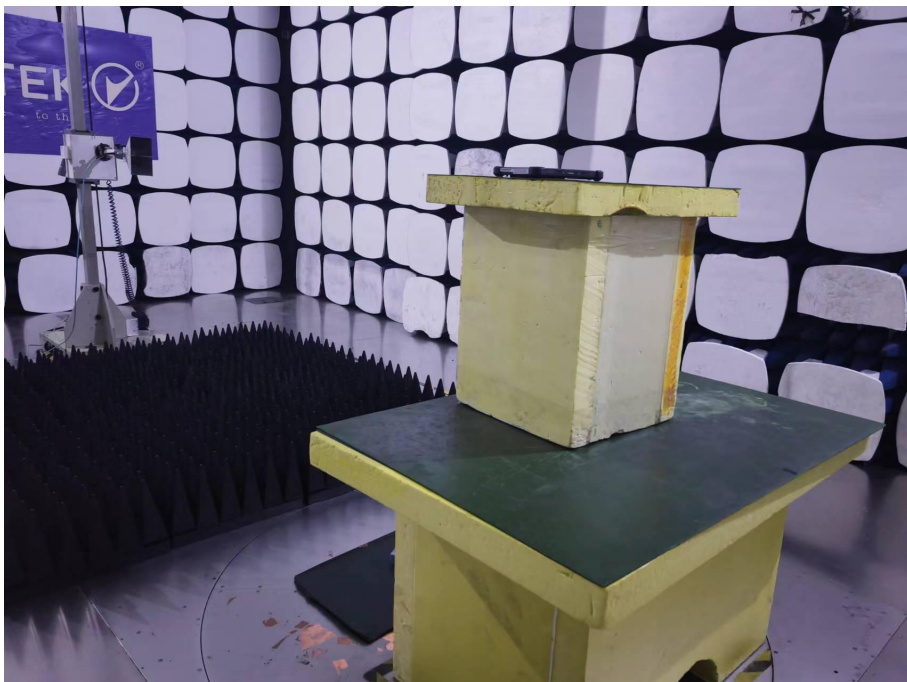
Spurious Emission Test Setup (Above 1GHz)
