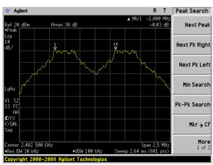
(1Mbps) Channel Separation plot on channel 00-01
