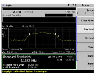
20dB Bandwidth plot on channel 78 (3Mbps)
