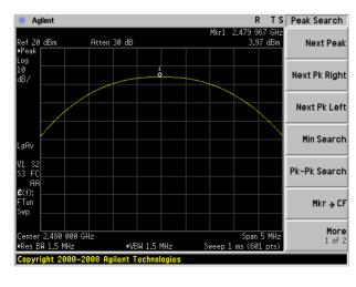
Peak output Power plot on channel 00 (2Mbps)
