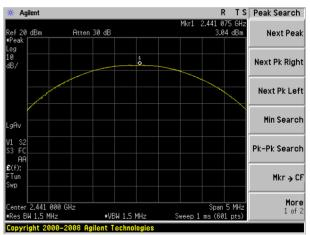
Peak output Power plot on channel 78 (2Mbps)
