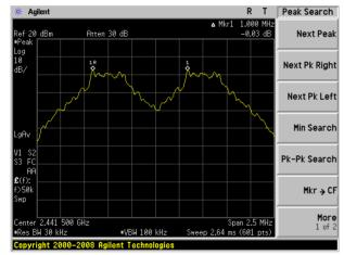
(1Mbps) Channel Separation plot on channel 77-78
