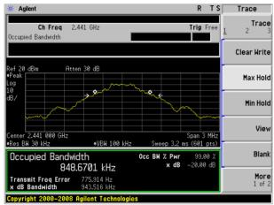
20dB Bandwidth plot on channel 78 (1Mbps)
