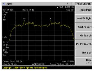
(2Mbps) Channel Separation plot on channel 39-40
