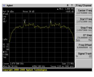
(1Mbps) Channel Separation plot on channel 39-40
