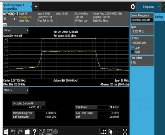
Band7-5MHz-64QAM-21425-25RB#0
